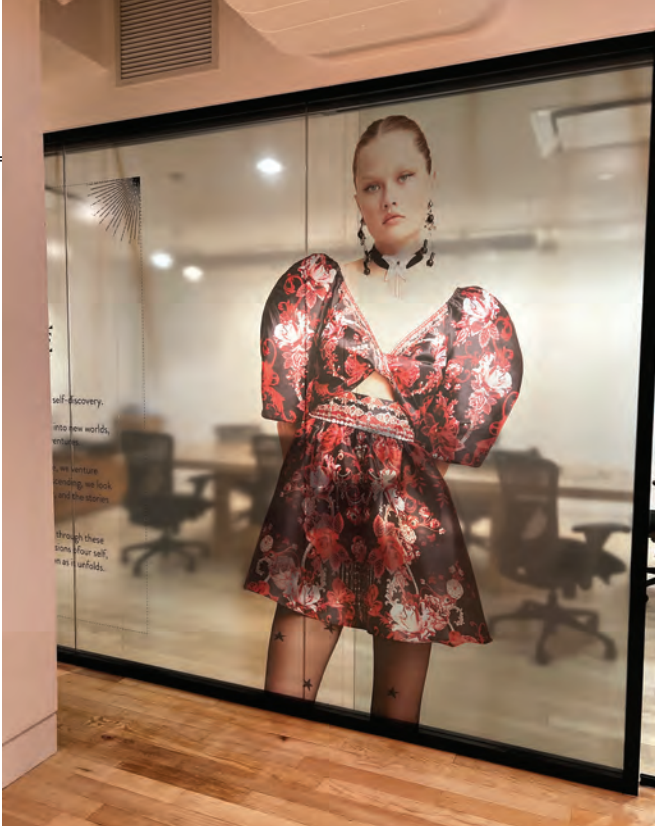
Example of translucent UV ink printed on clear film without white ink.
