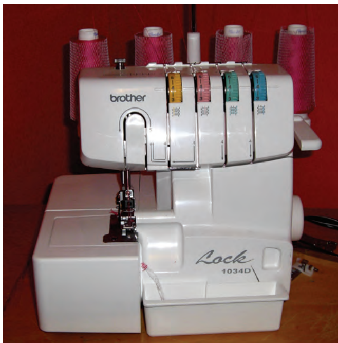
A serger is a type of sewing machine that can create a stitch with two, three or even four threads, and can also cut the edge of the fabric automatically to create a finished edge.
