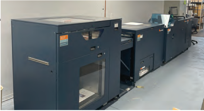
"Our Bourg is a high-speed booklet maker. Processes 700 books per hour." (Images courtesy of AlphaGraphics)
