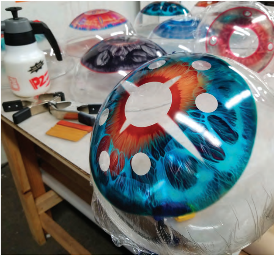
A high-density double-strike solvent print wet mounted to acrylic spheres.
