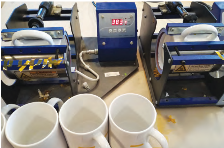
Any rigid item must be printed with transfer paper if it's to be sublimated, such as coffee mugs. (Image courtesy of Jennifer Foy)
