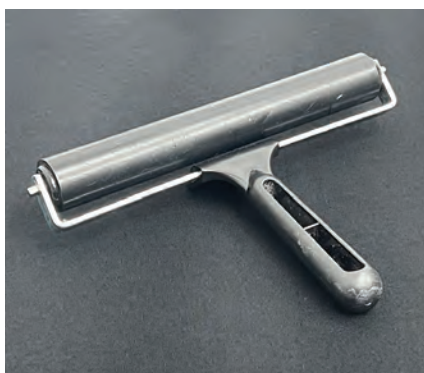
Using a clean and wide rubber print roller is an excellent method for achieving uniform pretreatment distribution before drying the shirt and has the added benefit of helping push down the shirt's fibers prior to printing.
