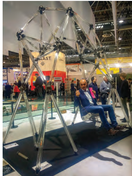
"The Swing" — completely constructed from Schott glass rods connected with 3-D printed steel nodes. As you can see, the structure supported the weight of an adult man.
