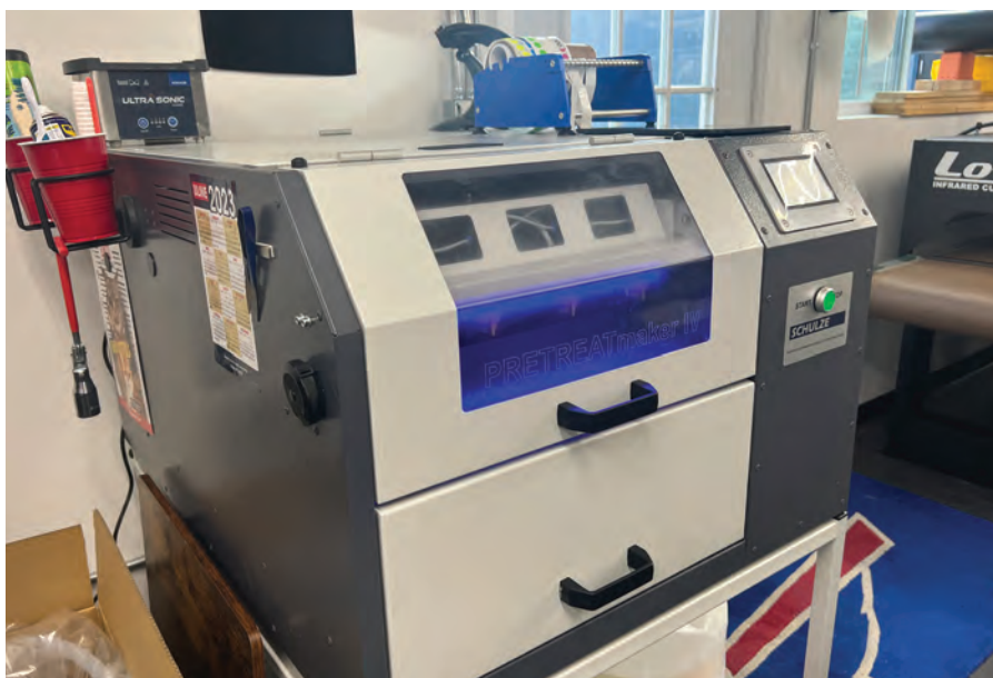
The Schulze PRETREATmaker IV allows us to pretreat shirts quickly and efficiently. Four spray nozzles ensure we pretreat only the area of the shirt we are printing with the correct amount of pretreatment solution.
