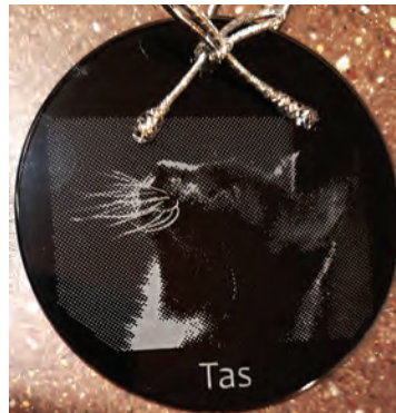
A 3" glass ornament with black background color, from Prism Products, gives splendid definition to photos etchings. The Letralight unit and Rapid Mask High Detail photo resist film, both from Ikonics Imaging, were used to create the stencil. The text was added using PVC sandblast resist material, cut on a plotter, and etched in a second run through the blasting cabinet.
