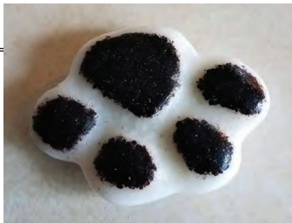
A cast glass Pocket Stone using a casting mold and glass frit, black fine grit for the pads, and white medium grit for the main body of the piece. Approximate size of finished stone is 2" x 1-1/5". The face of this cast glass paw is etched fairly deeply using Ikonics Imaging UltraPeel photoresist film for the design, and PVC sandblast resist for the name. Black paint was added for contrast.
