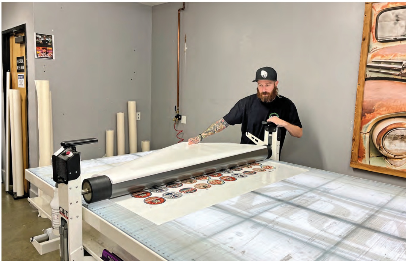
Mounting tables allow for more than just transfer taping. The ability to laminate short runs or test prints for customer approval allows us to maximize every inch of laminate laying around the shop.
