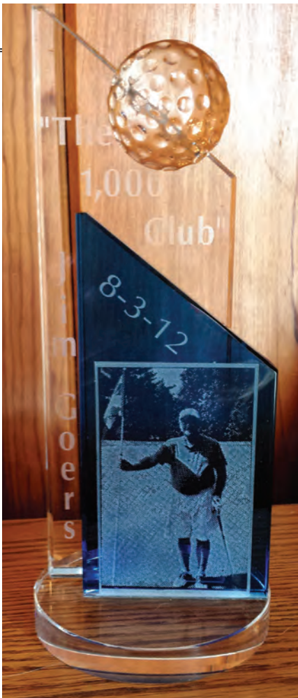
Golf-themed award blank, from Prism Products, surface etched with a photograph and text. Stencil materials used were Ikonics Imaging Rapid Mask High Detail, and 4-mil vinyl sandblast resist cut on a plotter, respectively.
