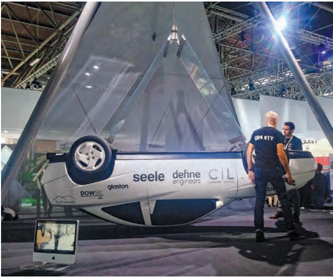
An upside-down car weighing 1.5 tons suspended from two panels of laminated glass no more than 4 mm thick. Who says that glass is fragile?
