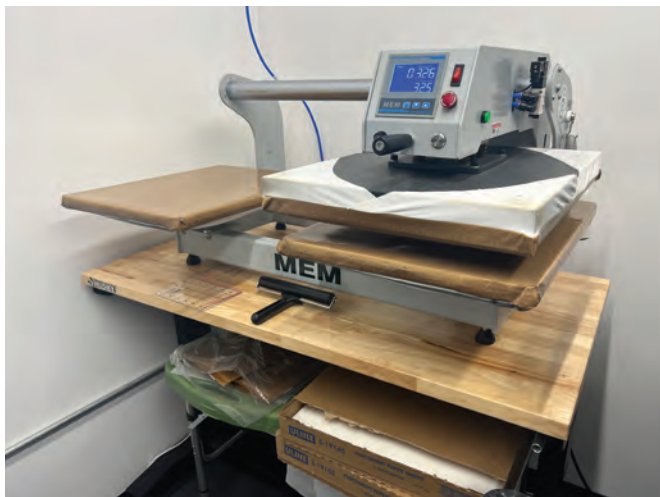
After pretreating shirts, a larger two-station pneumatic heat press dries the pretreated shirt and flattens the fibers of the garment to allow for an optimal print area.
