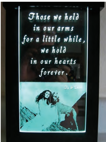
Custom built wall mount of wood with LED lights installed at the top. The 1/4" plate glass has polished edges, ground notches at the top for mounting, a photograph surface etched using Rapid Mask High Detail, and text deeply etched using a 4-mil vinyl custom cut stencil.
