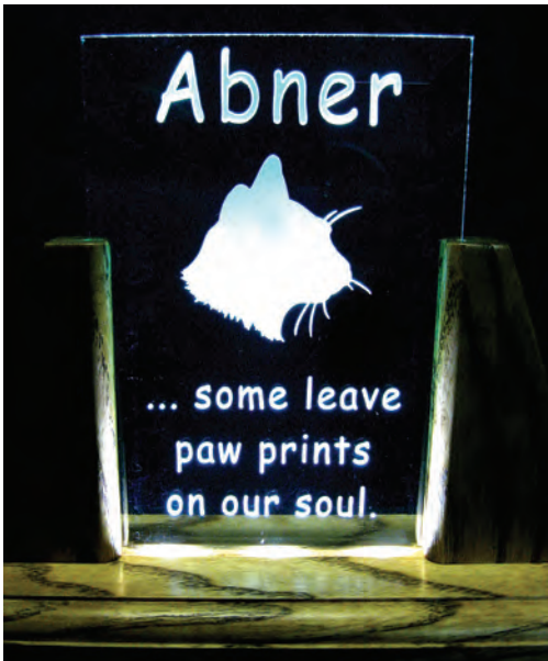
Custom designed and built frame with LED lights to illuminate the 4" x 6" x 1/4" crystal clear glass. A stencil plotter cut of 4-mil sandblast resist allowed a deeper etch to capture the light for this nightlight.
