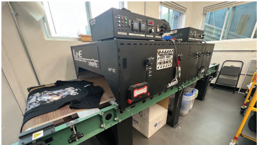
Our Vastex Lo-E Dryer cures our direct-to-garment prints without diminishing print vibrancy and maintaining a pace that matches the production speed of two printers.
