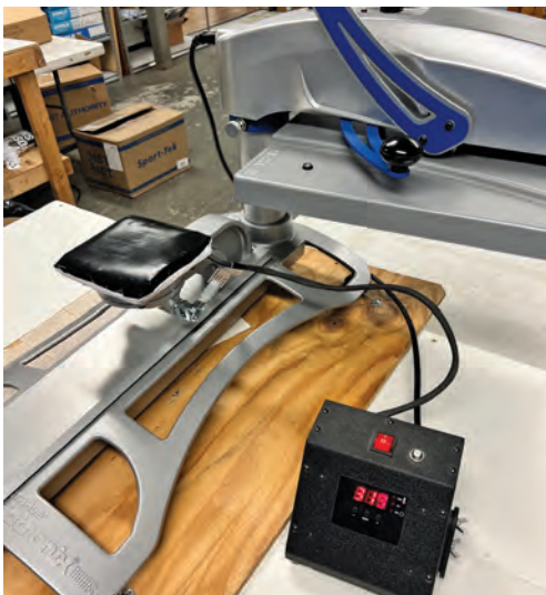
Smaller bottom heat platen. This particular unit is being used for cooler bags. Notice the bottom heat is reading 319 degrees (320 is programmed) the top heat is 280 degrees.
