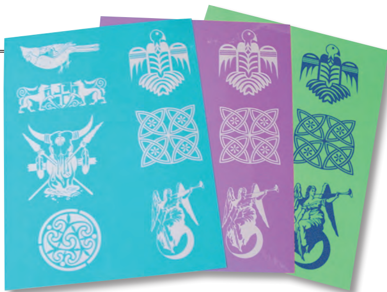
Various photoresist already exposed (imaged). The green resist is a non-washout resist and requires negative artwork instead of positive, as all others do. (Courtesy of Professor Glass)
