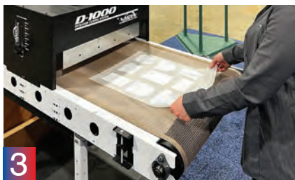
3 Set sheet into DTF compatible conveyor dryer with adhesive side up and cure for 60 to 90 seconds. Time and temperature may vary based on dryer manufacturer.
