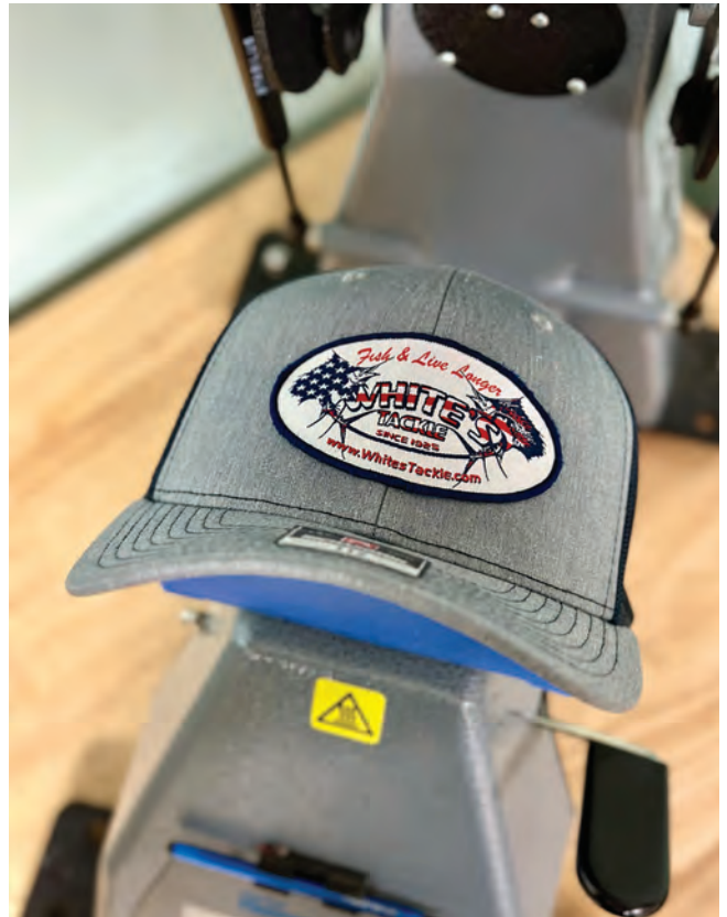
This structured hat has a patch with heat-activated adhesive backing applied with a hat press.
