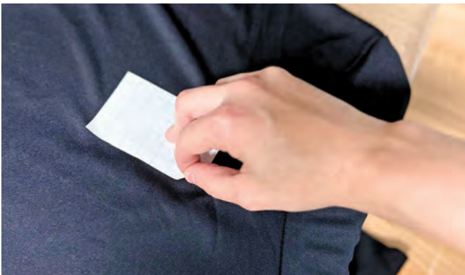
Polyester shirt gets a screen print transfer helping to avoid any potential off-gassing/dye-migration issues on press.
