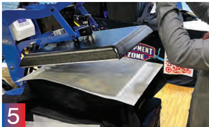
5 Heat press for ink/adhesive manufacturer’s recommended time and temperature. Allow shirt to cool down to room temp before peeling off the backing when using cold peel adhesive. When using hot peel transfer film, remove the backing as quickly as possible after pressing.
