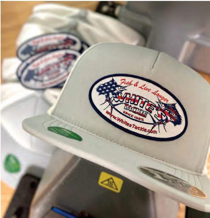
This foam hat has a patch with heat-activated adhesive backing applied with a hat press.
