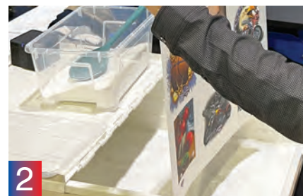
2 Repeat multiple times to get a nice consistent coating and shake off excess powder into collection system.
