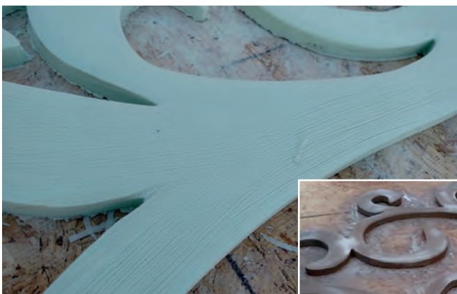
A CNC router was used to cut out the shape of the tree in 1" HDU while 1/2" and 1/4" pre-cut acrylic sheets had the gears nested into them and were laser cut.
