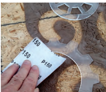
Sanding acrylic to prepare for paint, then spraying base coats of metallic colors.
