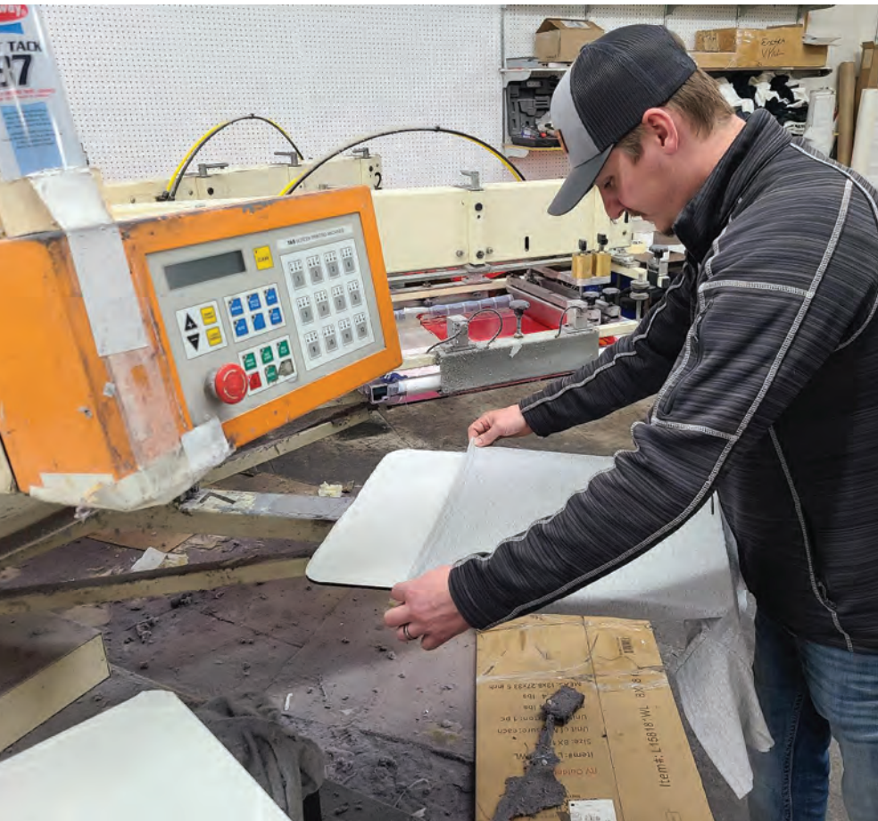
Ty Wilson printing on the automatic screen printer. That is where we would have printed the league logo on the front. (Image courtesy Nathan Craig)
