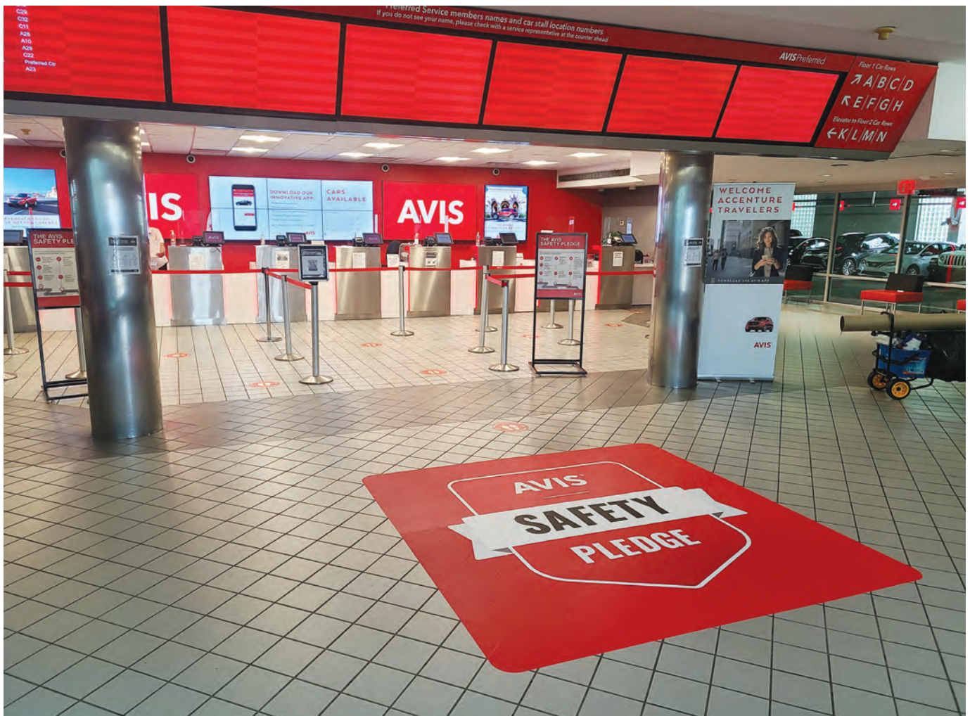
An example of using rounded corners to extend the usable life of the floor graphic.
