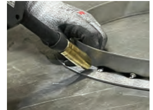
Photo 5A & 5B: Full retainer for channel letter on a bench in the shop. The return of the retainer is easy; routing the face takes skill and file management.
