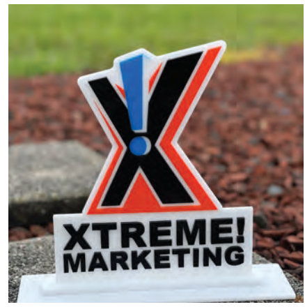
This sign is made entirely from pieces of acrylic cut on the laser, including the stand.
