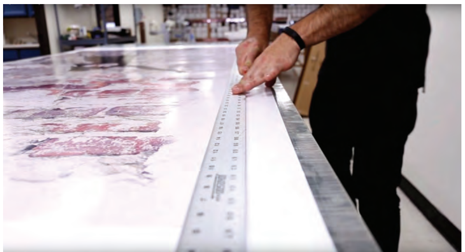
MetWest production team member trimming a custom printed Peerhatch wall covering panel.
