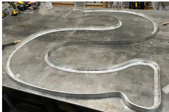
Photo 5A & 5B: Full retainer for channel letter on a bench in the shop. The return of the retainer is easy; routing the face takes skill and file management.
