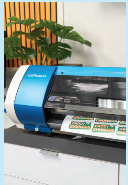
A series of Daddy Chungus logos for Scarcello's shirts being printed using Roland's VersaSTUDIO BN-20 desktop printer/cutter.
