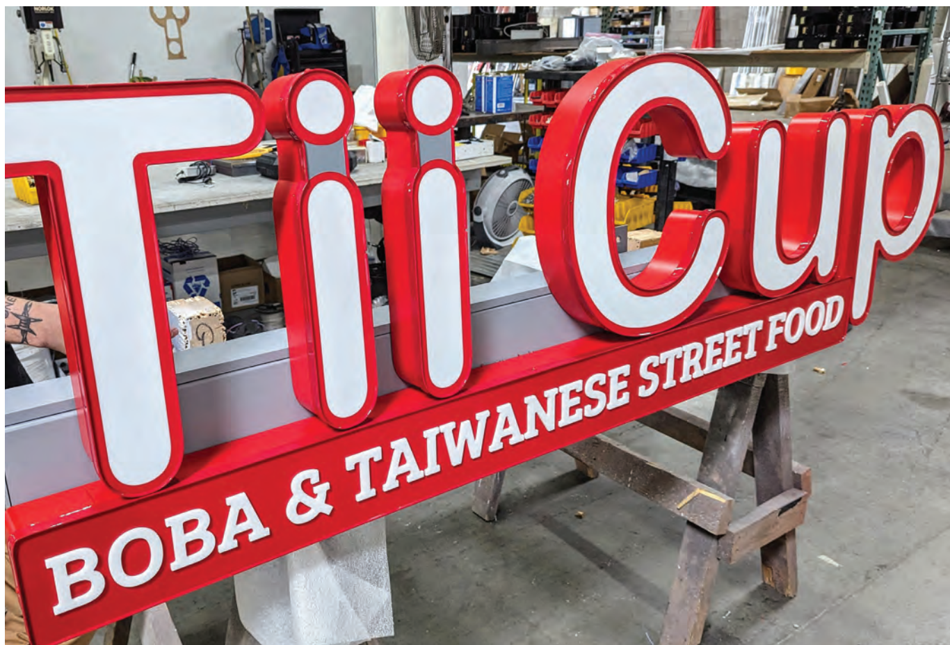
Channel letters are in high demand for the inside and outside of buildings that can either be front-lit or back-lit with LED lights.
