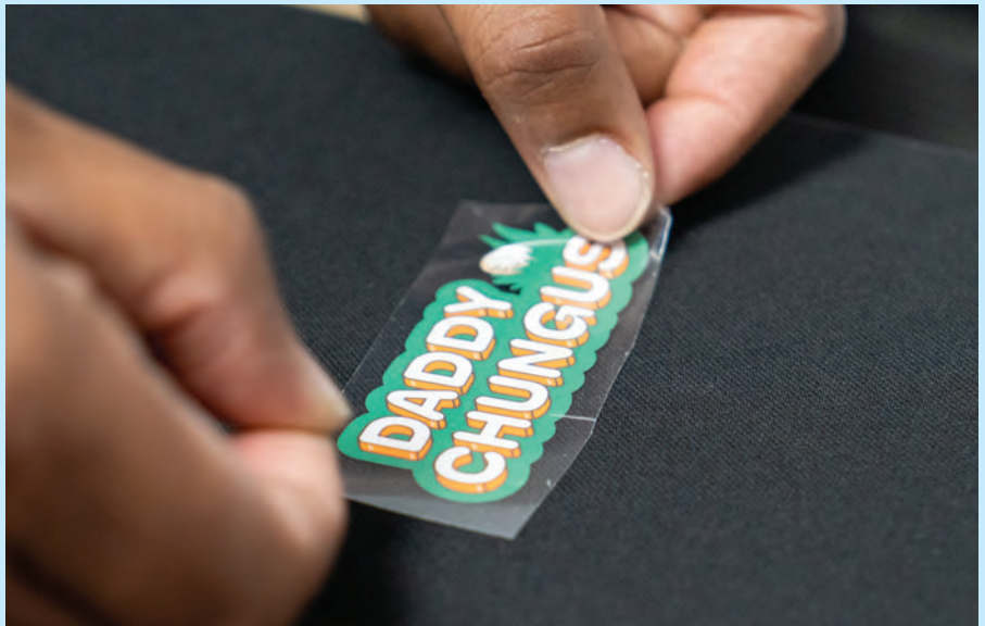
Scarcello's signature Daddy Chungus logo being prepped for transfer onto a shirt. The logo was created with Roland's TrueVIS VG3 printer/cutter.
