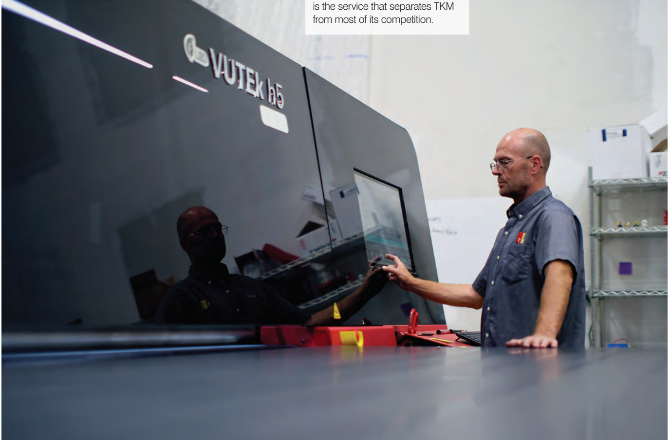
The company’s new EFI VUTEK H5 can print over 30 full 4x8 sheets an hour, four times the capacity of the original machines.
