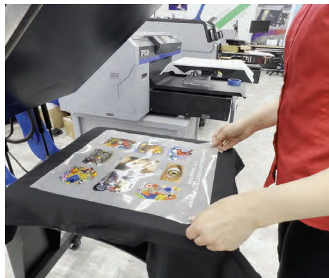
DTF transfers can be applied using either a clamshell or swing away heat press.
