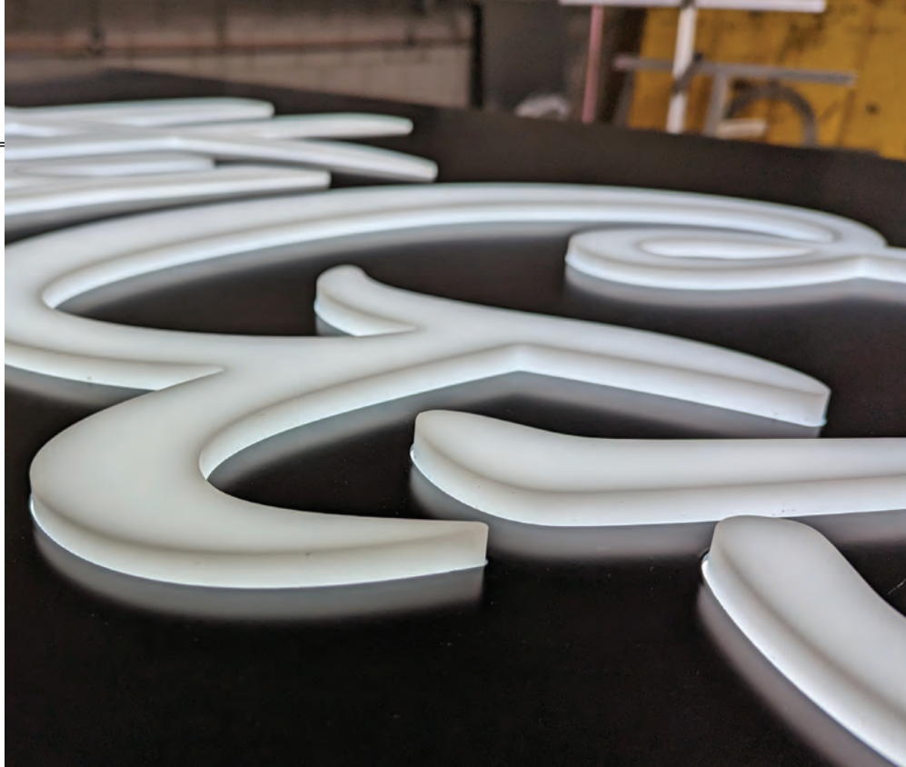
When routing half-inch acrylic, a shop will get a poor edge finish if the bit is not perfectly sharp.
