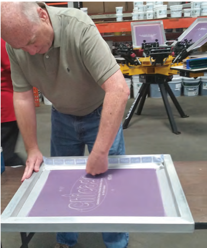
Taping the inside of the screen will help avoid ink leaks and speed up the cleaning process after production.
