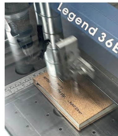
Dialing in a fairly fast speed and mid to low power is essential for cork.
