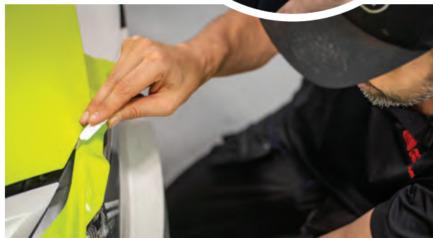
Wrapping a white car with a darker or bright color film requires more film for door jams, under the hood, and other areas so that the white paint will not be visible. Justin Pate demonstrates the proper technique for trimming film under the hood.
