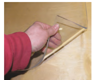
A cutting mat that provides a smooth, clean surface for cutting vinyl graphics. (Image courtesy Yellotools)
