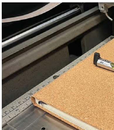
Check that the journal is level in the laser.
