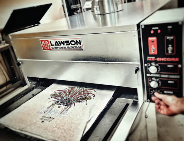
The conveyor dryer available from Lawson Screen & Digital Products is used to dry a garment after printing. (Image courtesy Lawson Screen & Digital Products)
