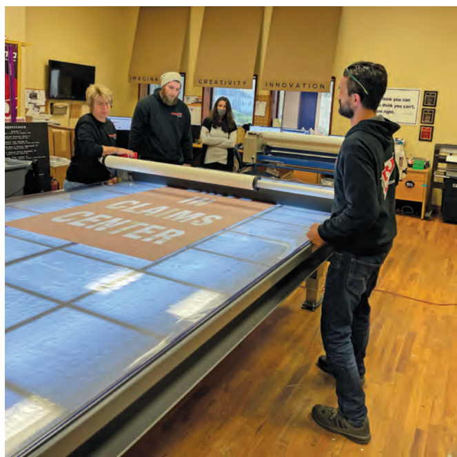
Signarama’s employees use the table to mount masked vinyl and digital prints onto various substrates. (Image courtesy Signarama Huntington Station)
