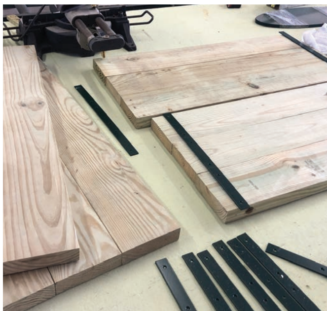
The flat bar metal trim at the end is merely decorative, as internal threaded rods actually hold the boards together.
