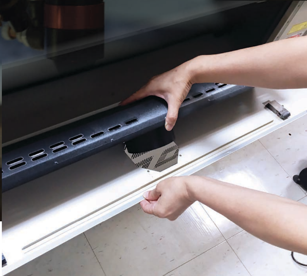
Maintain your machine's ventilation efficiency by cleaning the exhaust duct regularly.
