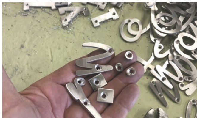
All metal parts were drilled and countersunk and buffed clean for powder coating.
