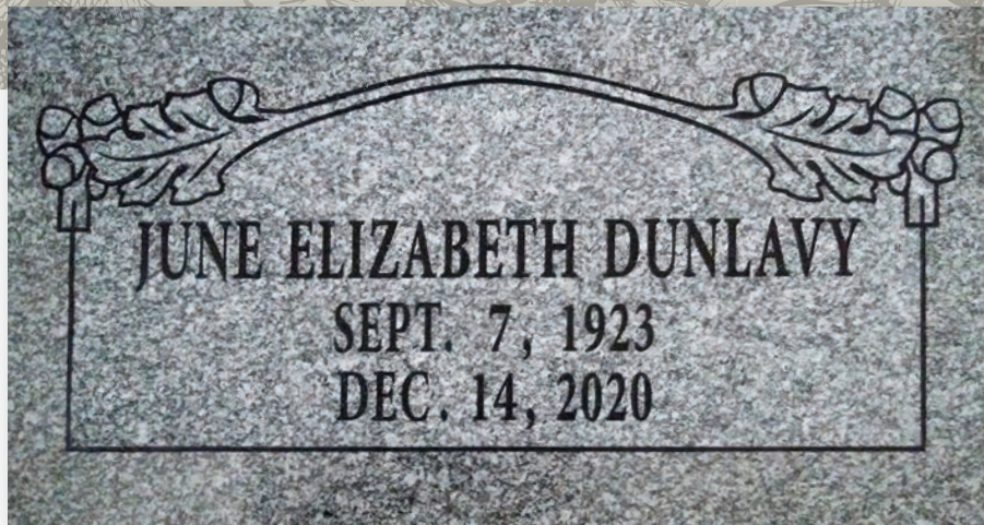
Left: A gray granite stone, abrasive blasted and filled with black paint for contrast. Below: Another type of green urn made from paper-like, environmentally friendly fiber products, which will deteriorate over time.
