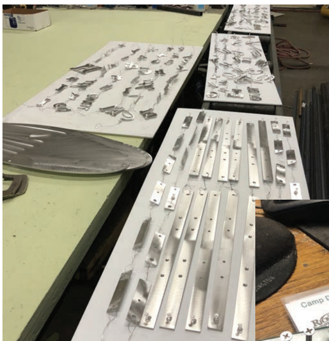
Above: To help hang these many small parts for powder coating, several items would be daisy chained together with electric fence wire. Right: Before sending parts to the powder coating shop, more than 300 stainless steel screws were put in a holder so they could be coated to match.
