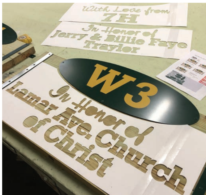
Perfect install patterns were cut on our laser and secured in place with push pins.
