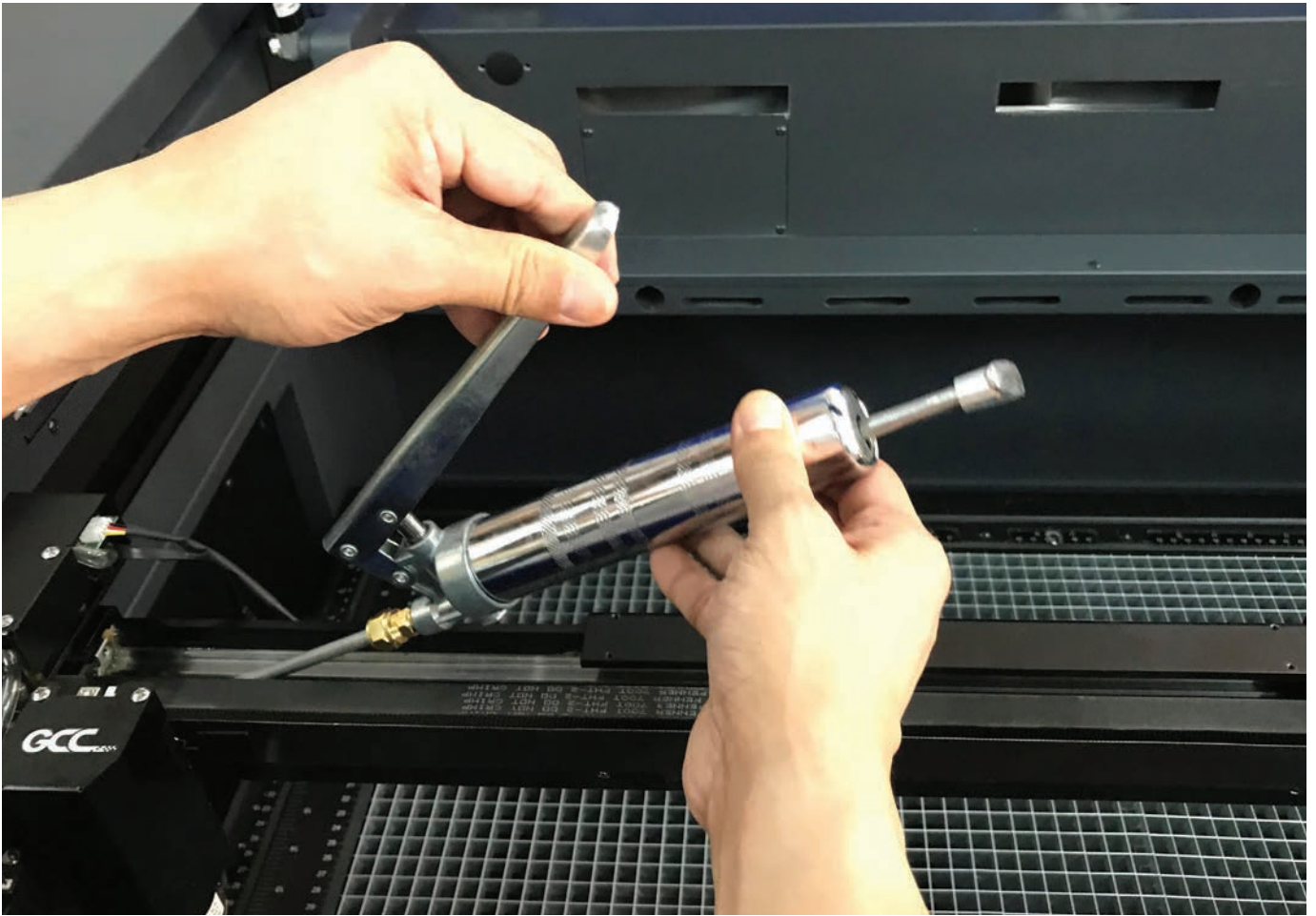
Too much oil or NSK PS2 grease applied to the Y rails accelerates debris buildup.
