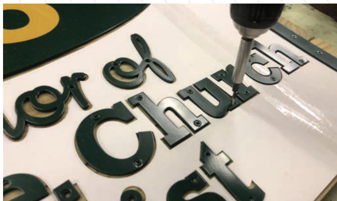
Matching powder-coated screws were recessed into countersunk holes in all our metal parts.
