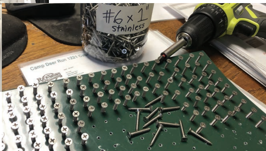
Above: To help hang these many small parts for powder coating, several items would be daisy chained together with electric fence wire. Right: Before sending parts to the powder coating shop, more than 300 stainless steel screws were put in a holder so they could be coated to match.
