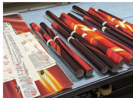
Most graphics arrive in a tightly wound roll, so it's important to lay them out, check for damage, cut down spot graphics, and roll and label panels for installation.
