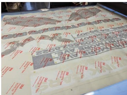
Most graphics arrive in a tightly wound roll, so it's important to lay them out, check for damage, cut down spot graphics, and roll and label panels for installation.
