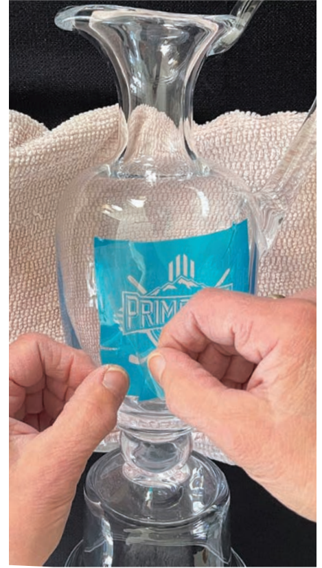
Applying the stencil with the cut pleats, peeling the cover sheet, and folding down the stencils at the pleats.
