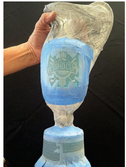
The completed blasted vessel ready for cleanup.
