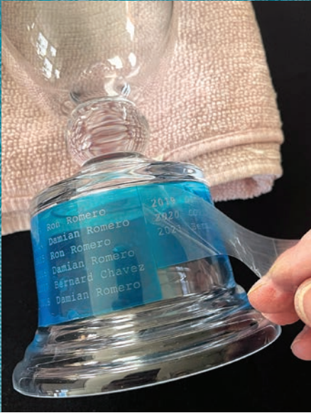
Left: Application of the base stencil with the names and peeling the cover sheet. Center and right: Taping the gap on the base stencil and the pleats.
