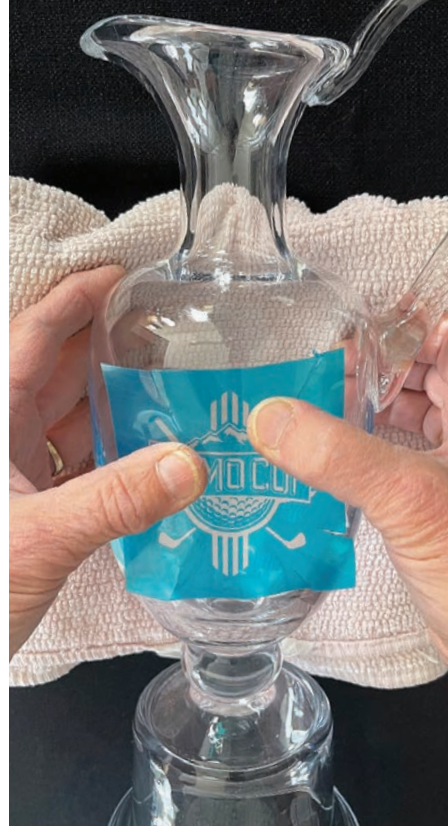
Applying the stencil with the cut pleats, peeling the cover sheet, and folding down the stencils at the pleats.
