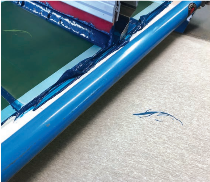
We started with unbased dark blue on a 230. Wanting a clean opaque print on heather, our first down white screen would go on 156 TPI (thread per inch), both stretched to 30 N/cm perpendicular and parallel on work hardened retensionable frames.
