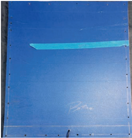
Place the backing panel onto the frame and pre-drill holes for fastening.
