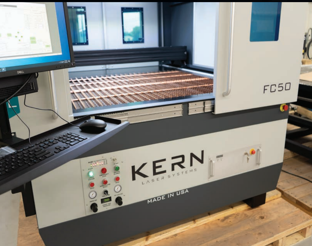
With a large-format laser, material loading and unloading is performed less often due to the large sheets the machines can accommodate. (Image courtesy Kern Laser)
