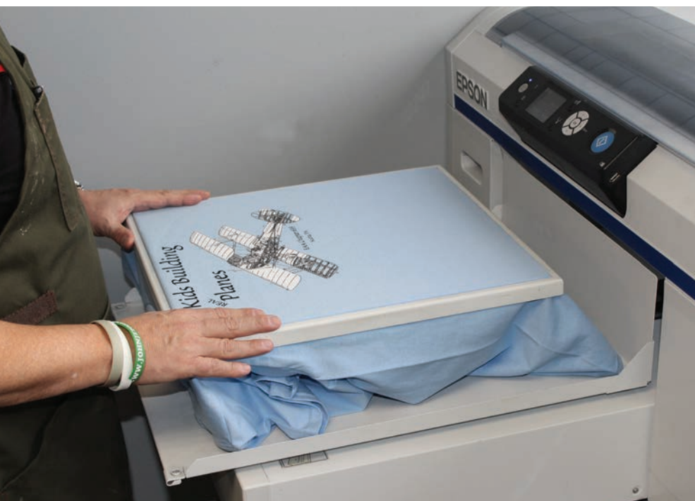
Top: An employee of Shirt Pickle loads a T-shirt onto a printer for DTG printing. Above: Shirt Pickle prints an image onto a T-shirt using the DTG printing process. (Images courtesy Shirt Pickle)
