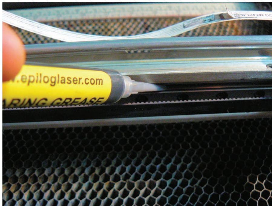
Lubricate rails on schedule, as provided by the manufacturer. Do not over lubricate.
