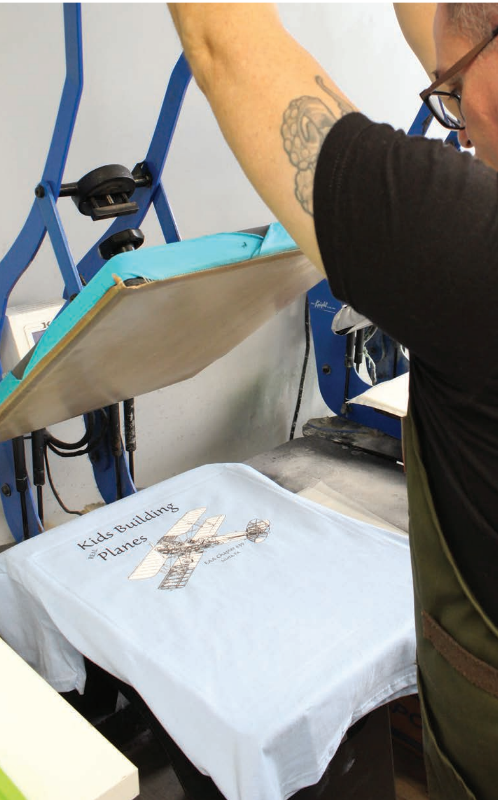
A Shirt Pickle employee uses a heat press to cure a DTG print. (Image courtesy Shirt Pickle)
