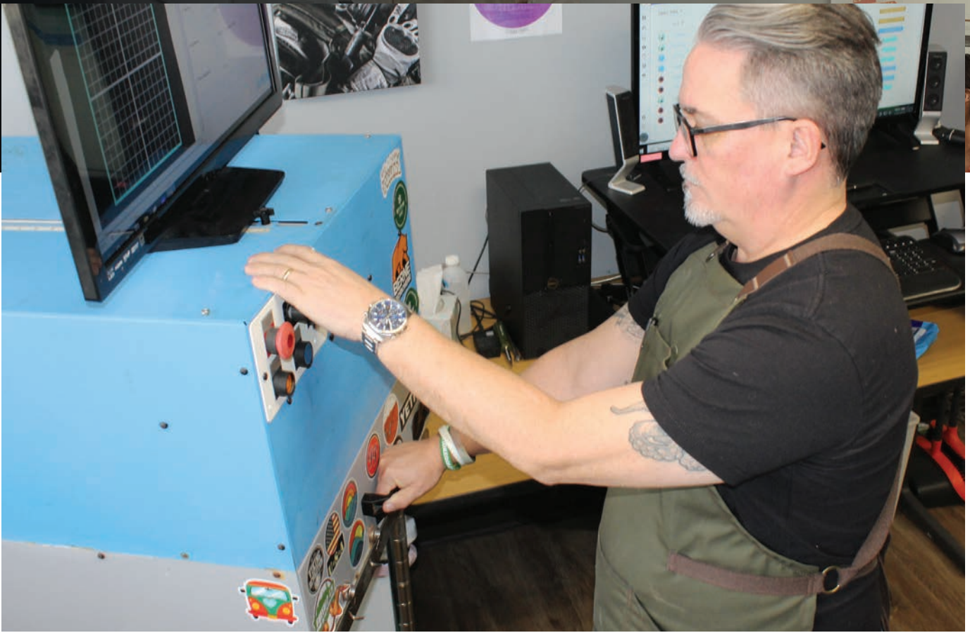
An employee of Shirt Pickle pretreats a T-shirt to prepare it for a DTG image. (Image courtesy Shirt Pickle)
