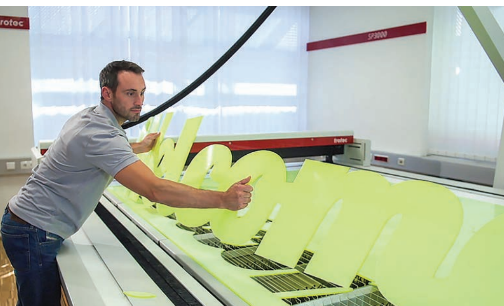
Above: Large-format lasers are typically offered in higher wattages for thicker material cutting. (Image courtesy Trotec) Right: Shops can make the most of their large-format investment by taking advantage of the size and capabilities. (Image courtesy Trotec)
