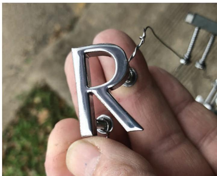
This "R" is a sample of one of the smallest sets of real metal letters we've ever had to work with. The size was only 1.25" tall by .25" thick and was actually stud mounted.
