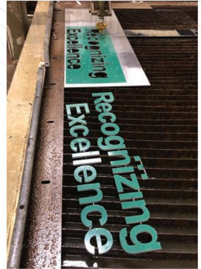
**Left:** To protect our sheet from piercing scuffs from waterjet cutting, the material was temporarily covered with vinyl, but this step was likely not needed. **Right:** The set of letters was waterjet cut, and then we had to remove the protective vinyl.
