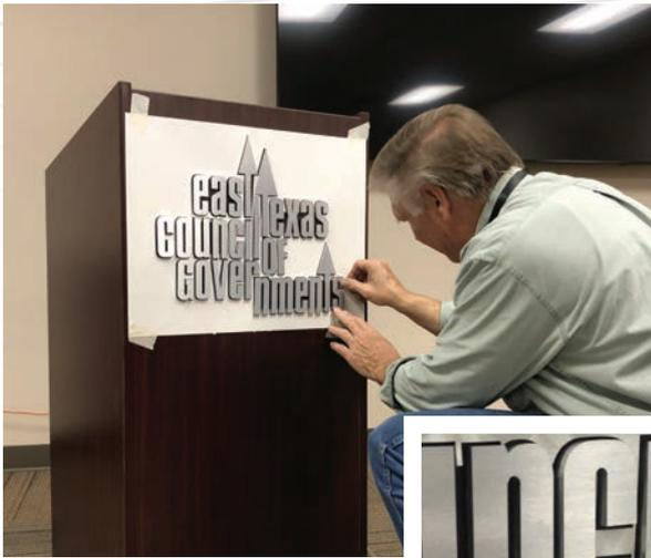
**Right:** Double-sided foam tape, plus very small drops of clear silicone, are used to adhere our faux “brushed aluminum” lettering to the front of the podium.
