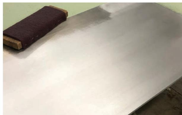
was put in the letters with the same board covered in Scotch-Brite, by merely dropping each letter back in the hole where it came from, and several firmer strokes on the faces of each letter made the straight grain brushed metal finish a bit more visible.
