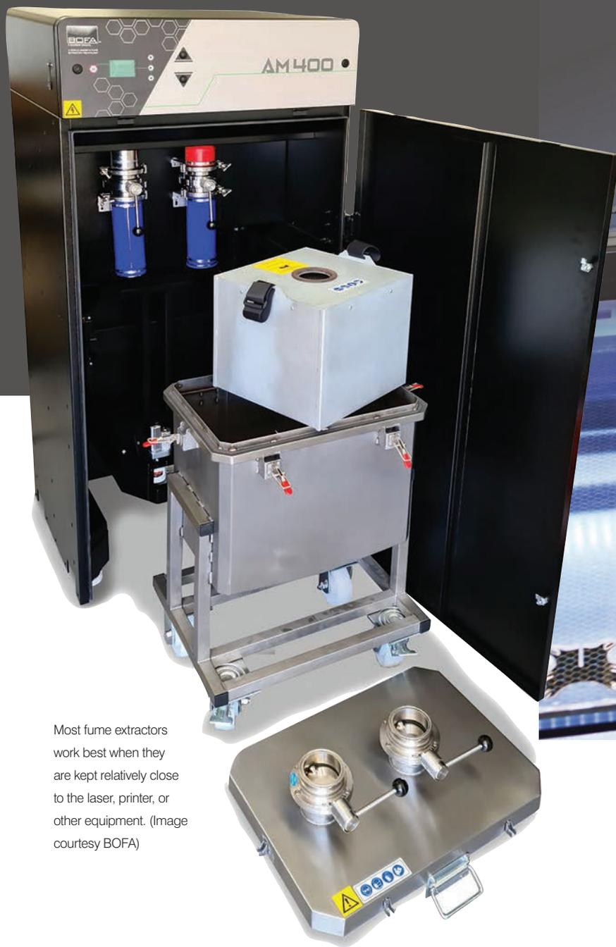
Most fume extractors work best when they are kept relatively close to the laser, printer, or other equipment. (Image courtesy BOFA)
