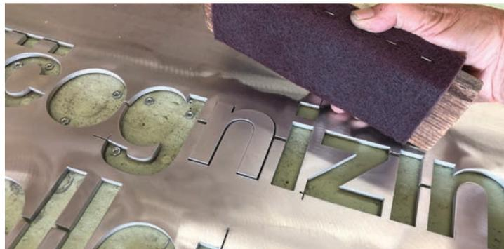
The letters were held stationary by dropping in the matching voids in our scrap material. Very small nuts were set in the holes to raise each letter above the surface of the sheet.
