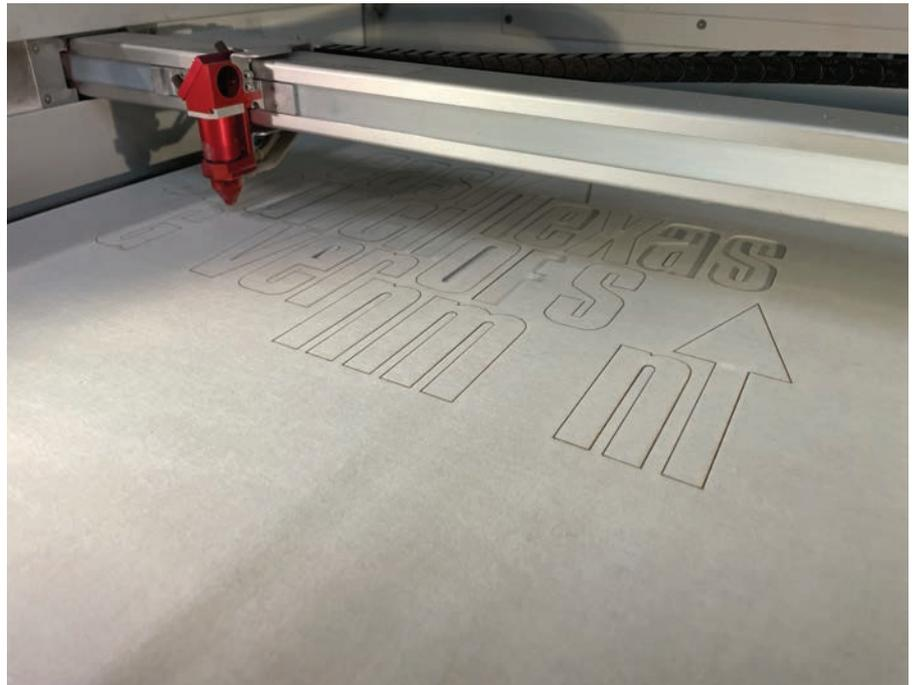
The transfer tape used to apply the sheet of film is left on while the laser does its work.
