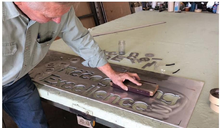
The final grain was created from making several straight-line strokes with our Scotch-Brite block, while applying firm downward pressure.
