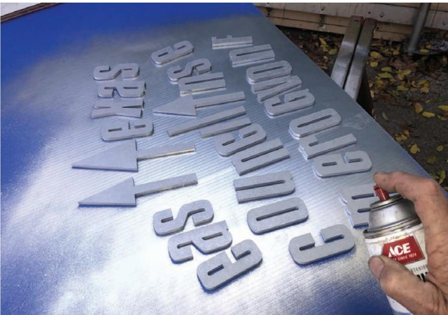
With the transfer tape still on each part, to get the edges to look like aluminum, the edges are given a light but overall coat of aluminum colored spray paint.
