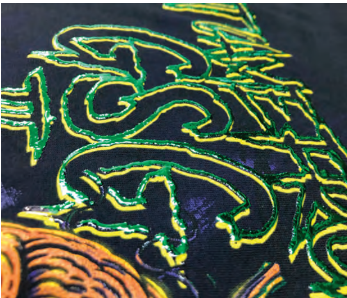
The clear was also used as an adhesive for foil added for the area of the text "It came from GSG II."
