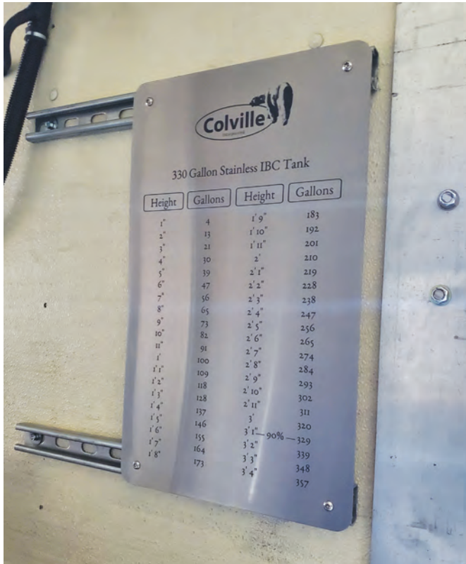
Hatch printed a strapping chart onto a stainless-steel panel that can be mounted on a wall of a lube truck. A strapping stick with inch gradations is used to determine the number of gallons of fuel.
