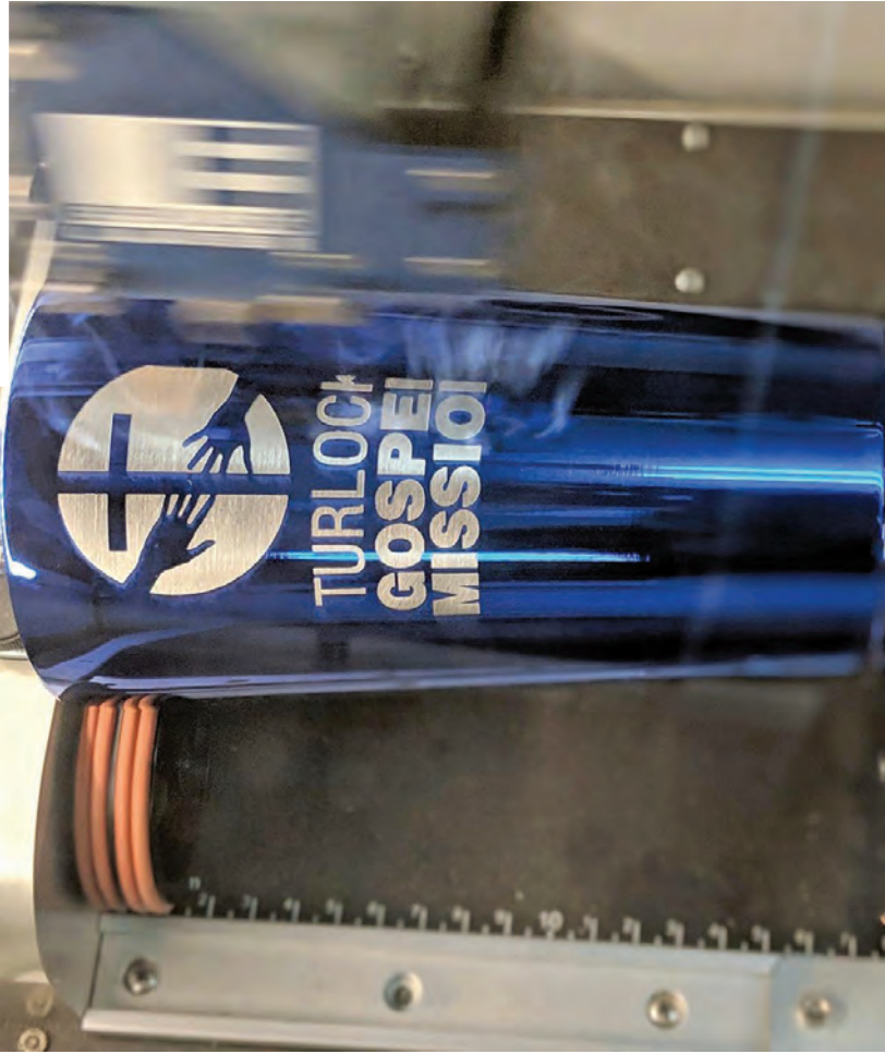
Rotary attachments and specialized products like CerMark spray improve the engraving process.
