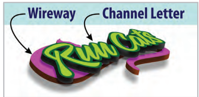
Photo 1: A typical example of a logo after being redrawn as a set of channel letters on a raceway. The cat head is the icon of their logo. (The raceway is pink in this example for clarity of detail only) The basic raceway option involves an enclosed box that can be fabricated or an extruded raceway, with a water-tight lid or a hinged face -- or it can be stick-built with an internal framework for larger, heavier letter sets. It's typically used when the letter set is simple, budgets are low and the client or landlord want's simplistic consistency with all of the tenant's channel letter signs.
