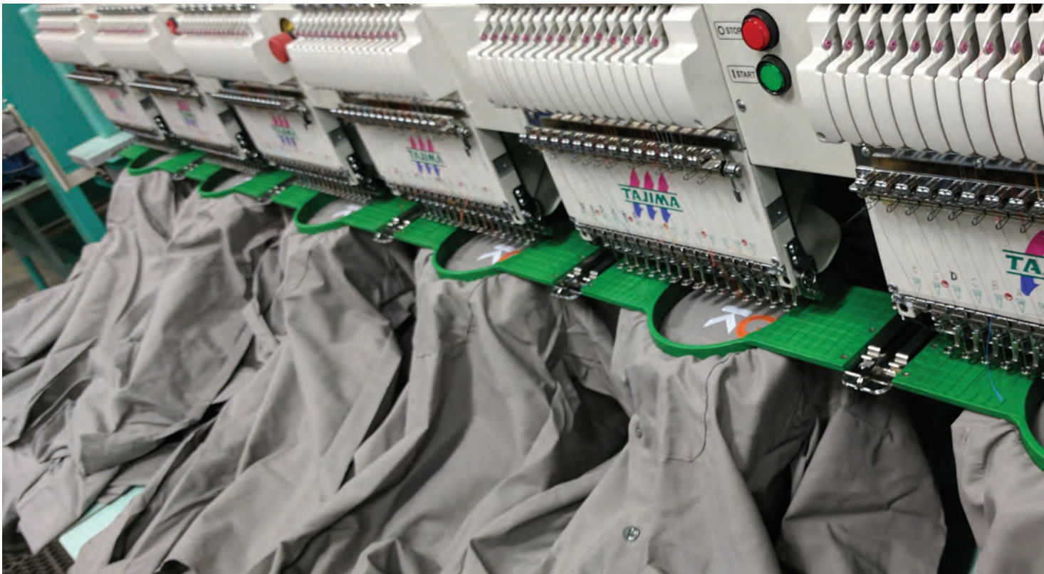
A run of uniform shirts on a multihead machine. (All images courtesy Erich Campbell)
