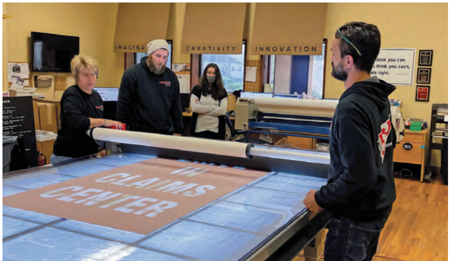
Signarama’s employees use the table to mount masked vinyl and digital prints onto various substrates. (Image courtesy Signarama Huntington Station)
