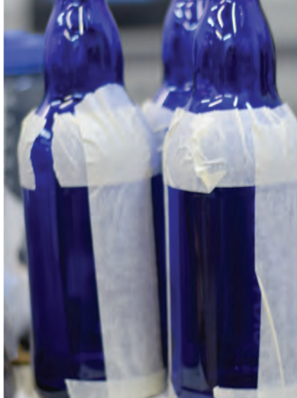
Step two of the sandcarving process. Once your design has been placed, it is time to mask off the glass.
