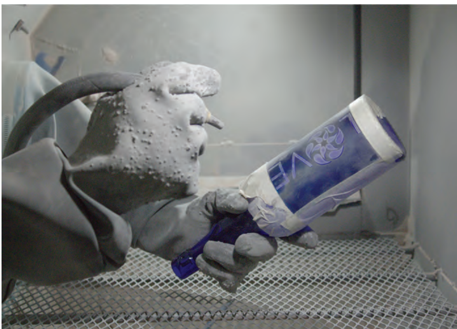
When blasting, it is crucial for your nozzle to remain 90 degrees to the surface of your piece.
