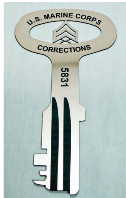
The large jail cell key was laser cut from a 24" x 12" sheet and laser engraved.
