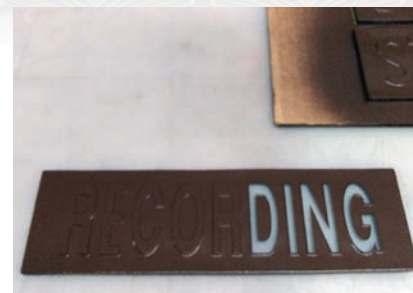
Left: Beginning to peel off the stencil, showing that the side wall of the letter is painted. Right: Peeling the stencils letter by letter.
