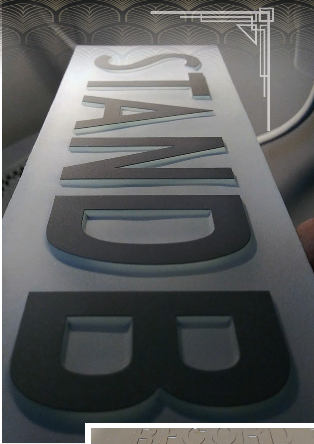
Above: Showing the depth around each letter. Right: A set of signs covered with the brown paint.
