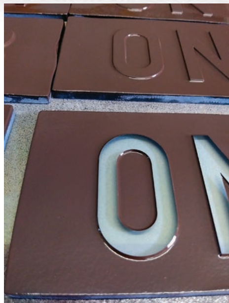
Left: Beginning to peel off the stencil, showing that the side wall of the letter is painted. Right: Peeling the stencils letter by letter.
