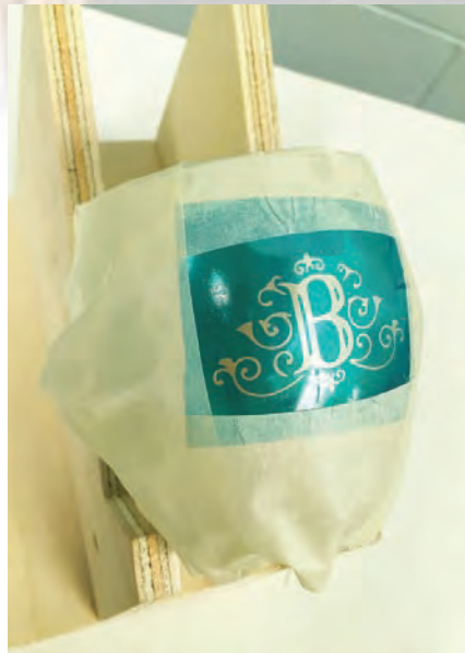
Photoresist masks are used for flat, curved, convex, or concave surfaces. (Image courtesy IKONICS Imaging)
