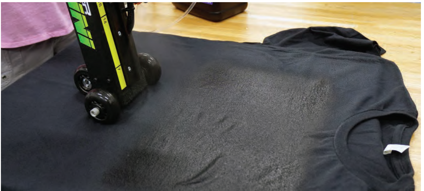
A hand-controlled pretreatment machine spraying a shirt; pretreating correctly is a big issue to overcome. (Image courtesy Brian Walker)
