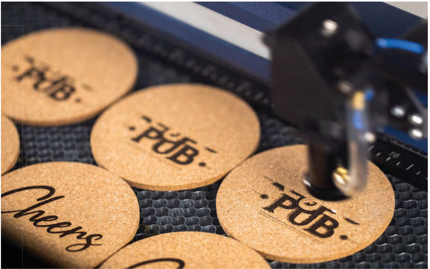
With high-volume laser equipment, you can set up an entire table full of products to be engraved in one run. (Image courtesy Epilog Laser)
