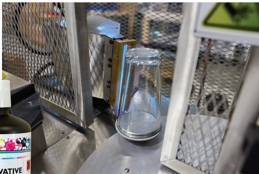
Above: A view of the dual flame and Pyrosil treatment by the PYROBOND 4 GL System. Left: An example of an adhesion promoter that would be hand-applied prior to printing. (Images courtesy Michael Perrelli)
