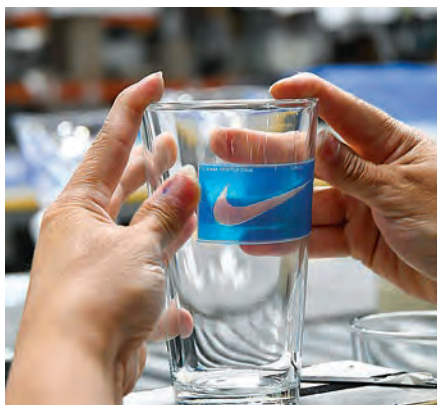
The mask application process is dry and only requires a clean work bench. It is essential to have good lighting as this helps with accurate mask alignment, especially on curved or convex surfaces. (Images courtesy St. Regis Group)
