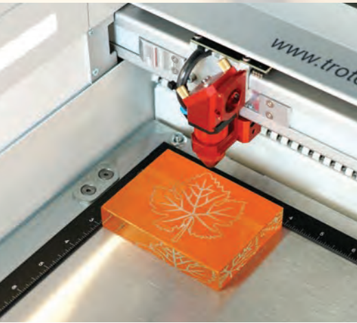
Laser masks are normally used for flat surfaces. Laser masks do not have quite as crisp lines as a photoresist mask does, but they eliminate the develop and washout steps. They've become popular due to many shops already using CO 2 lasers. (Image courtesy Trotec Laser)
