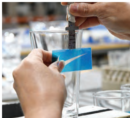
The mask application process is dry and only requires a clean work bench. It is essential to have good lighting as this helps with accurate mask alignment, especially on curved or convex surfaces. (Images courtesy St. Regis Group)
