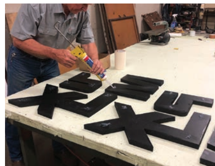
Clear silicone is used as an adhesive to secure our stud mounts in place.
