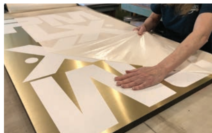
Plotter cut vinyl templates were cut using paint mask vinyl and applied to our metal-faced sheets, paying attention to the orientation of the brushed aluminum pattern.
