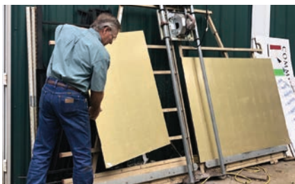
The first step, after acquiring a full 4' X 8' of this UltraBoard Aluminum material in a 1" thickness, was to cut the sheet down to just the size our two new logos would require.
