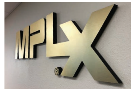
This photo shows one of two custom logos, hand cut from 1"-thick sheet, and then stud-mounted into the wall in about 30 minutes' work onsite.
