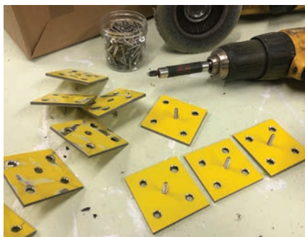
A small, sharp screw is threaded in place, and its head is countersunk so the pad remains flat for gluing.
