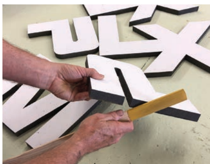
The sanding strokes are downward so as not to delaminate the thin metal surface.
