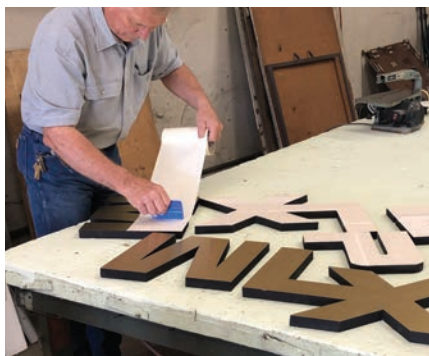
A new protective mask is applied using transfer tape, and carefully trimmed in place.
