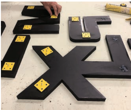
Only a few studs were required as all the parts are very light. The glue is allowed to dry overnight.
