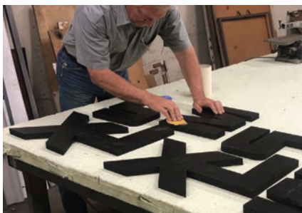
On the backs of our parts, the places where pads will be glued in place are scuffed up with sandpaper. The pads were scuffed as well.
