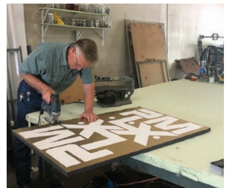
Each part would be rough cut first with a hand jig saw.
