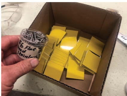
Our stud mount pads are made from small square pieces of scrap aluminum laminate and small #6 size stainless-steel sheet metal screws.
