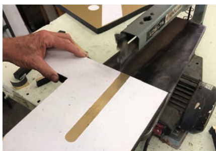
Our old scroll saw, equipped with a sharp fine-tooth blade, was used for all the cutting required. A smooth steady speed is required, not too fast and not too slow.
