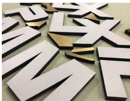
Here, all the parts for two logo displays are shown ready for sanding and painting the edges.
