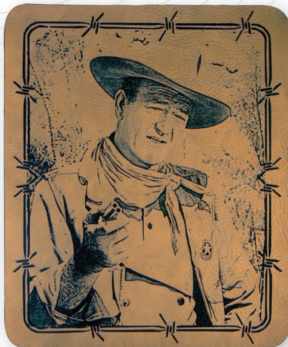
Above left: A leatherette plaque plate that lasers gold. There are a variety of sources for leather and leatherette products. The safest way to purchase them is from laser industry sources. Above right: This leatherette project was cut from a 12" X 24" sheet. Photos can be lasered, providing a unique and beautiful look.
