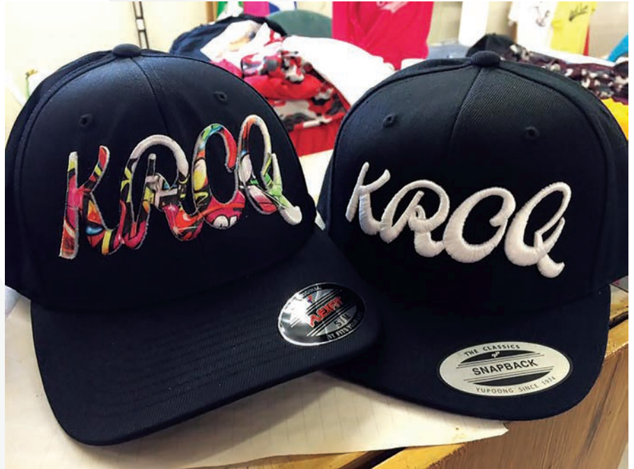
Two caps with identical embroidery couldn't look more different. The application of a sublimation print over white polyester thread on 3D foam makes for bold patterns and colors on this piece. (Image courtesy Tom Farr, Buzzard's Bay Embroidery)
