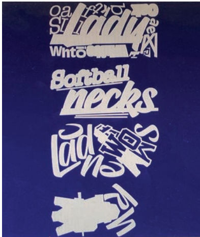
Four sheets of .125 mill finish 5052 aluminum was required to supply this cut file.
