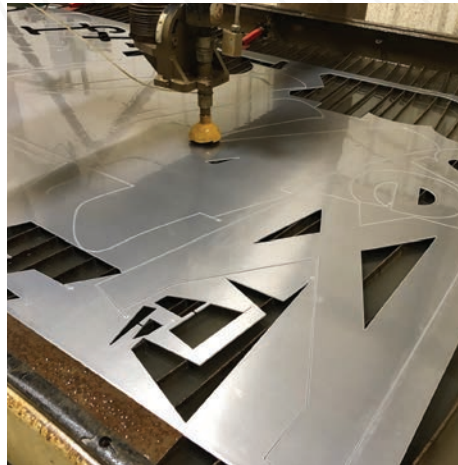
Our old waterjet, located across the street from the sign shop, made short work of these large aluminum cutouts.
