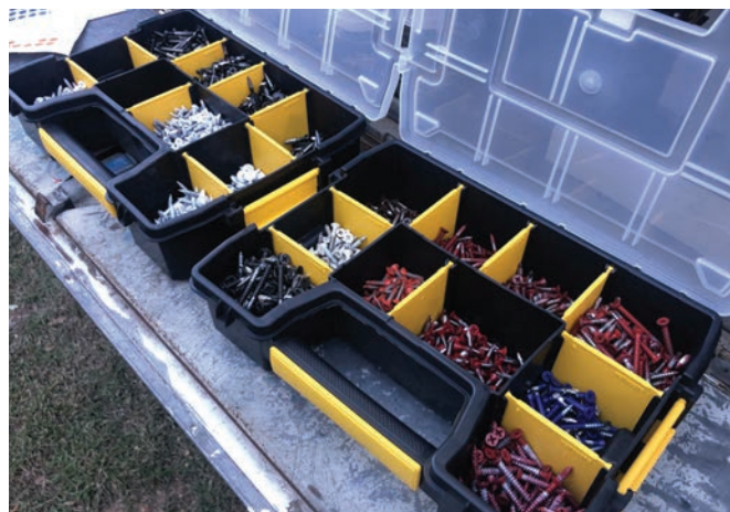
All the screws used were stainless steel, and some were powder coated in advance.
