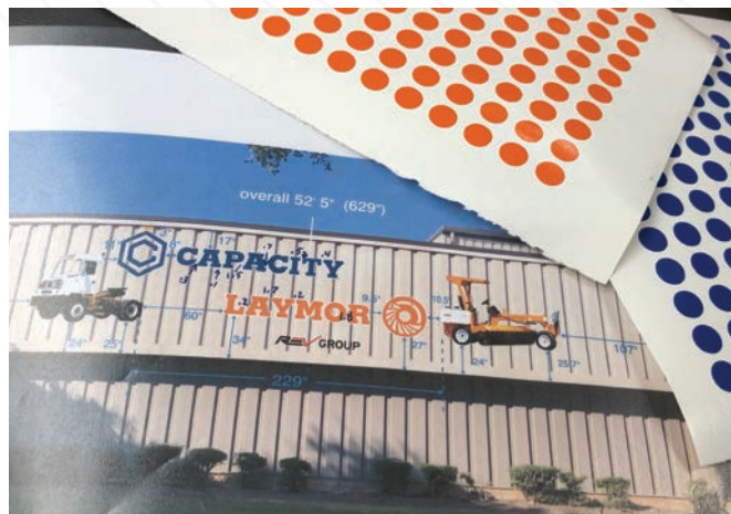
An accurate image with plenty of measurements goes to the job, along with matching vinyl dots to cover some of the screw heads.
