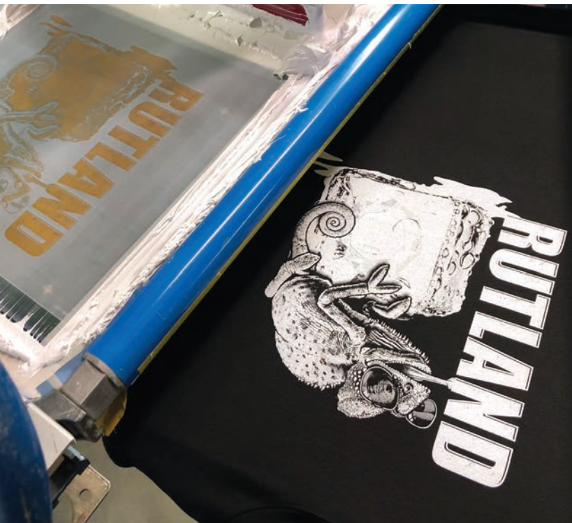
We ran the white on N-166 TPI screen at 45 N/cm2 using a 65/90/65 triple ply, dual durometer squeegee followed by a flash and smoothing heated iron in a Teflon screen.
