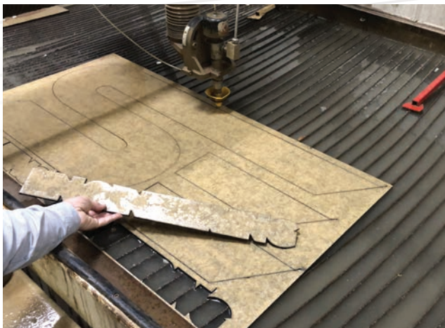
This logo, though made from acrylic, had to be cut on our waterjet because part of it was larger than would fit in our CO 2 laser.
