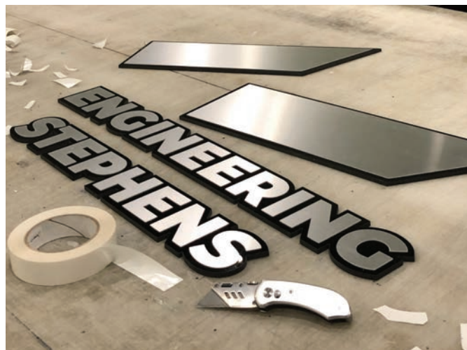
The 1/4"-wide margin around the metal parts provides a contrasting border for parts going on a gray weathered wood wall.
