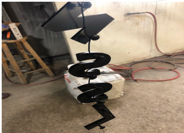
Some parts were hung for coating with hooks, others were daisy-chained together with small wire (like the ones in this picture).
