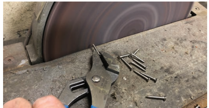
Small #8 screws with oversize heads would be put in the backs of each letter or logo part so parts could be hung for powder coating, but their sharp points were dulled a bit so they would not make protrusions on the fronts of the letters.
