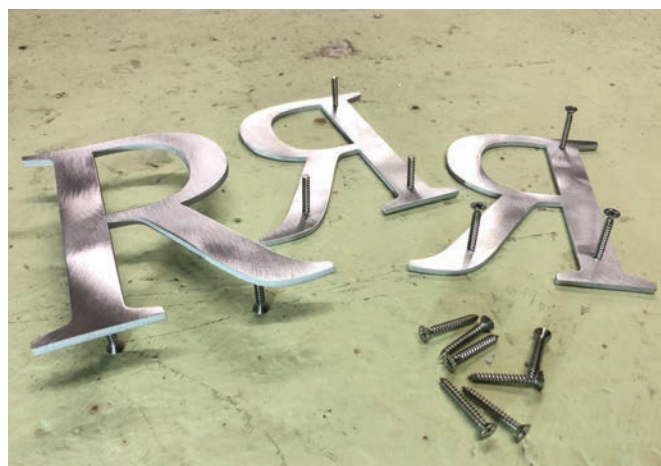
As an experiment, these three aluminum letters, only 1/8" thick, were set up for hanging for coating and potential "no hole" stud mounting, a real trick with .125" metal but possible. Dulling the points of the screws with sander or grinder first is a must.
