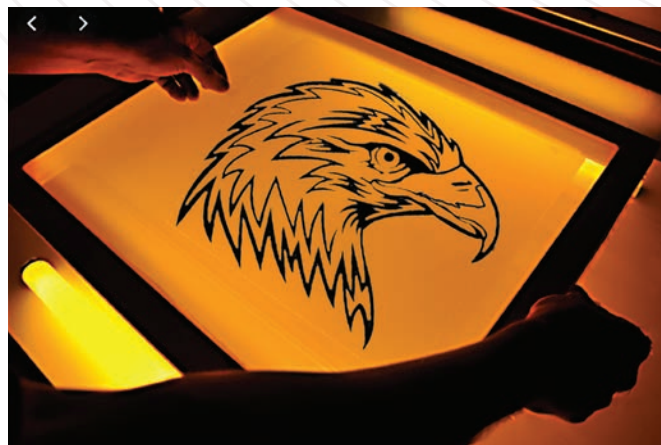
Figure 3. A film positive output from a computer onto a piece of transparent printable film.
