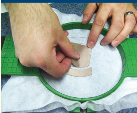
Using an adhesive, place the cut pieces on the stabilizer.
