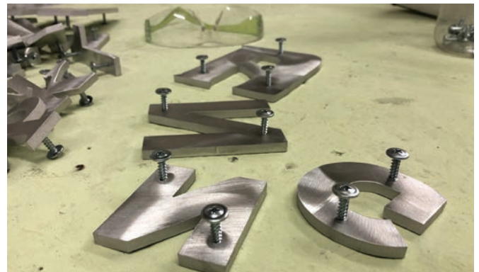
These buttonhead screws were chosen for hanging the letters for powder coating, since powder coat hooks won't slide over them.
