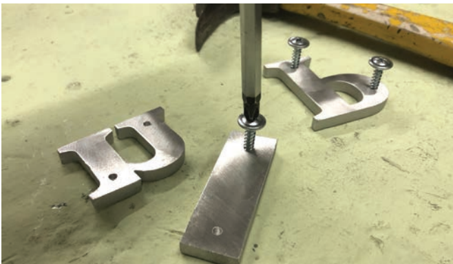
A light hammer tap on the screwdriver allows the screws to get a bite into the small holes on the backs of each part, and a simple half turn sets them firmly.
