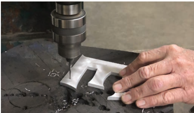
Instead of drilling threaded studs, typically 3/16 diameter, these parts were drilled with a small 3/32" bit and threading would not be needed.
