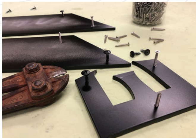
After coating, the buttonhead screws were removed, and smaller #6 size stainless screws were threaded in place to create micro-studs.
