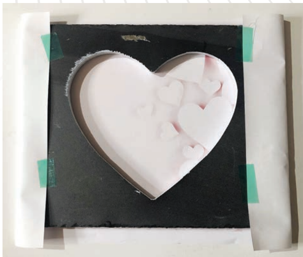
Step one of the sublimation process: secure with heat tape.
