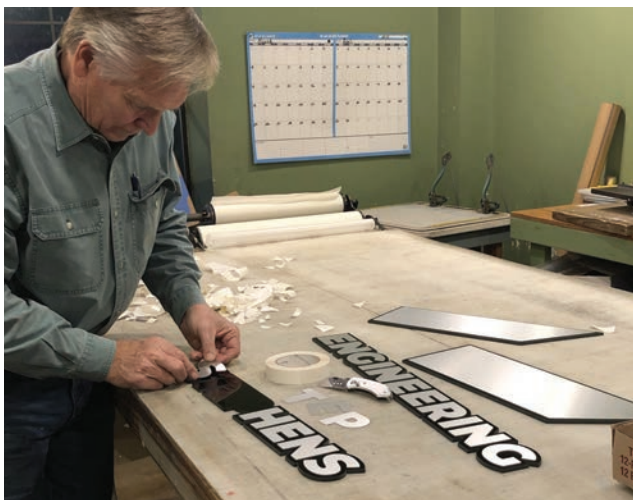
Double-sided tape is used to secure the metal parts to our acrylic components.
