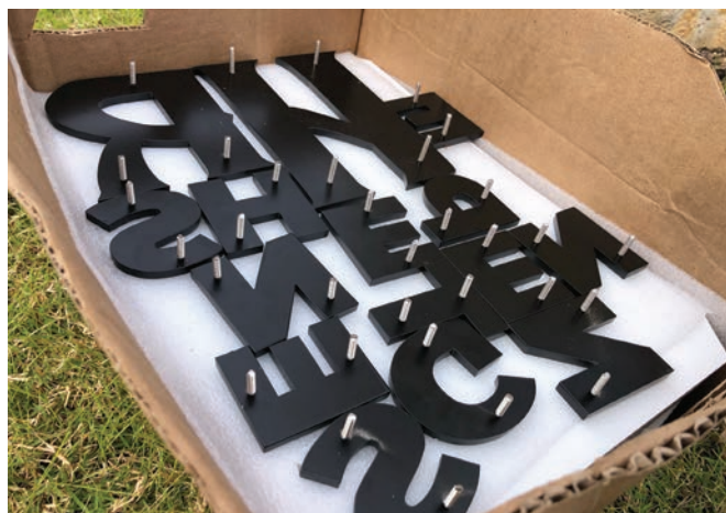
In this small box were several layers of studded parts with corrugated plastic sheets placed between layers.
