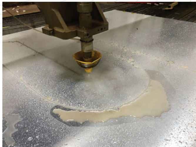
Cutting the thin (.040) brushed aluminum overlay parts on our old Omax waterjet.
