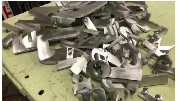
The exterior logo parts and letters were all cut from .25"-thick plate aluminum and were prepared for a special version of stud mounting.
