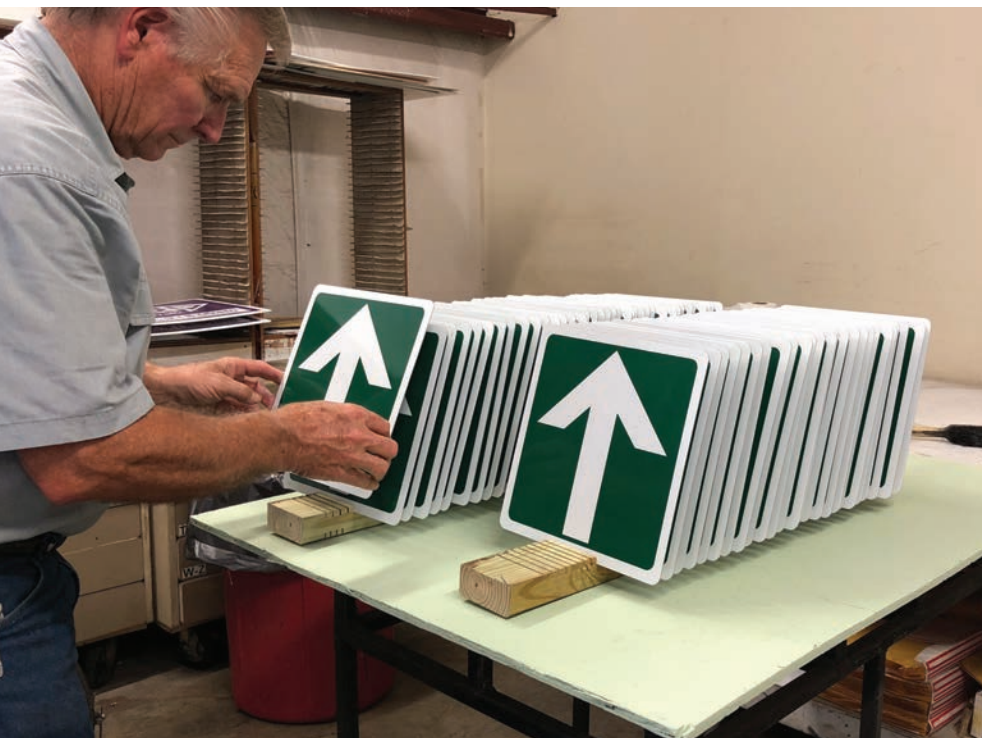
Another screen job done with a template for double-sided printing — 80 double-sided arrow signs done in short order and made to last.
