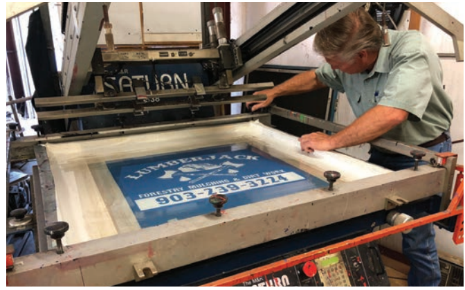
We have had an M&R clamshell press for more than 30 years, and it is often used to print corrugated plastic signs.
