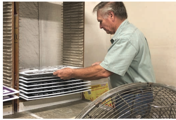
With a fan moving air over freshly printed signs, at least in warm weather, the signs are dry enough to turn over and print the backs in one printing run.
