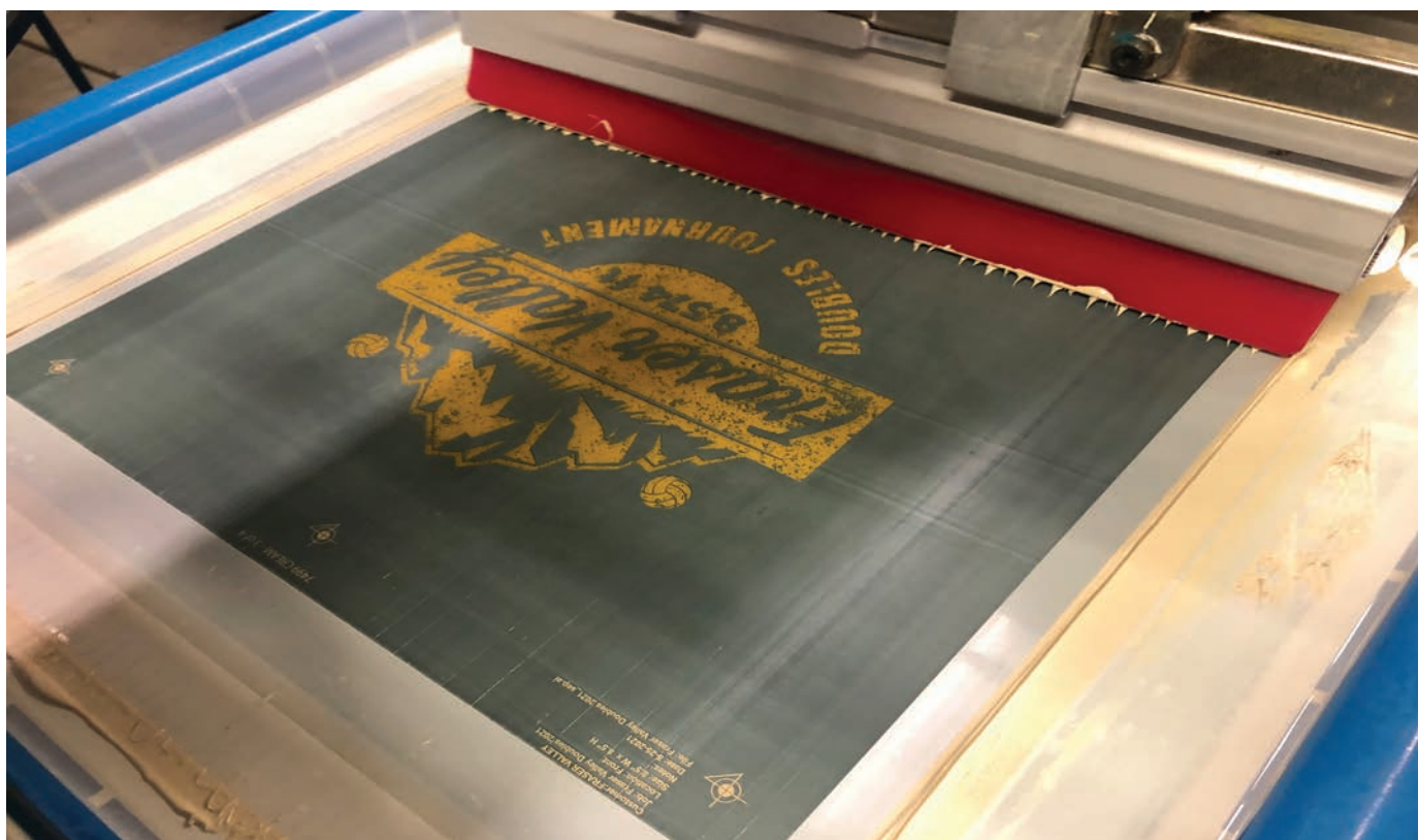
The colored inks ran wet on wet on 272s at 45 N/cm, using all 65/90/65 triple-ply, dual-durometer squeegees.
