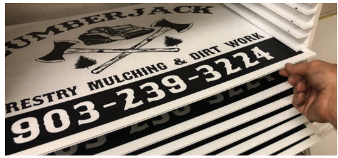
This simple shop-made drying rack was created with scraps of MDO, strips of fluted plastic, and small finish nails.
