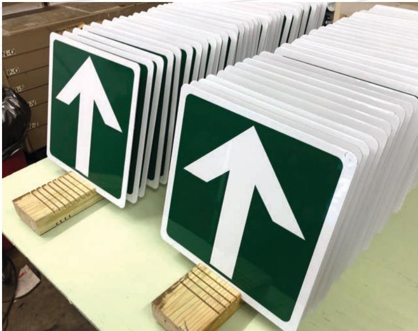
Above: The grooves in our "drying racks" merely needed to be shallower than the margin of white space on these arrow signs. Right: Signs we most commonly screen print are spot color corrugated plastic signs for contractors, politicians, and special events.
