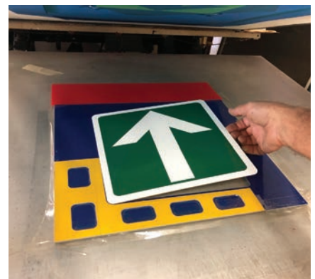
The jig is registered to the image in the screen and taped in place. The front side is printed, then flipped over and the back gets printed without delay.
