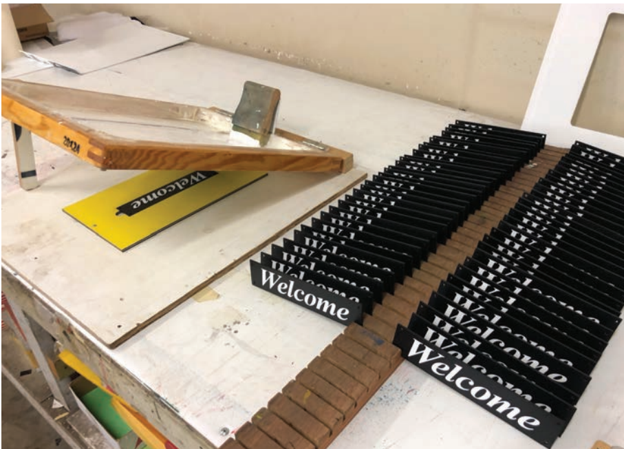
A small wooden screen, hinged to a scrap of MDO, with a kick leg to hold it in the "up" position. This setup is about as simple as it gets for screen printing in the sign shop, and this arrangement has been used many, many times. (All images courtesy the author)
