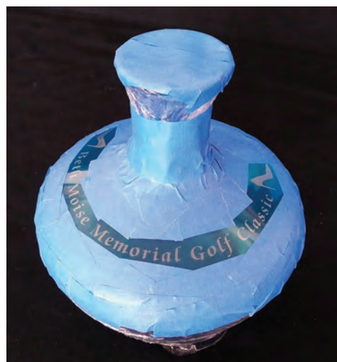
The stencils applied, and the decanter covered with shrink wrap and tape ready for blasting.
