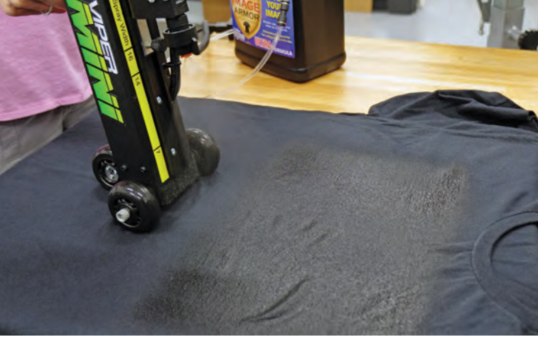
A hand-controlled pretreatment machine spraying a shirt; pretreating correctly is a big issue to overcome. (Image courtesy Brian Walker)
