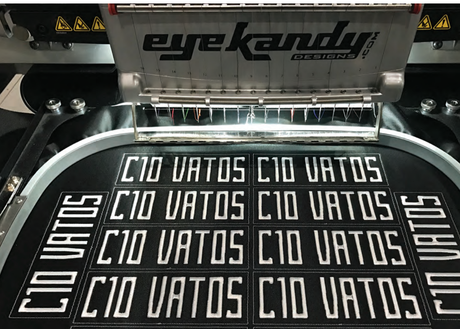
These patches were created using the applique-style method, stitched without edging and manually cut from a span. (Image courtesy RJ Silva, Eyekandy Designs)
