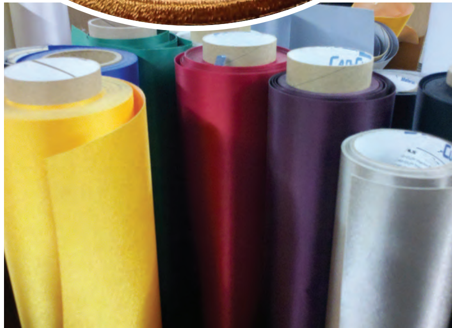
Though you can use almost any sufficiently stable fabric for patch-making, the classic choice is a polyester twill. (Image courtesy Erich Campbell)
