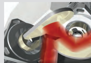
A galvo system is different from a gantry system because instead of moving a large lens over the work piece, the system uses moving mirrors to deliver the beam.
