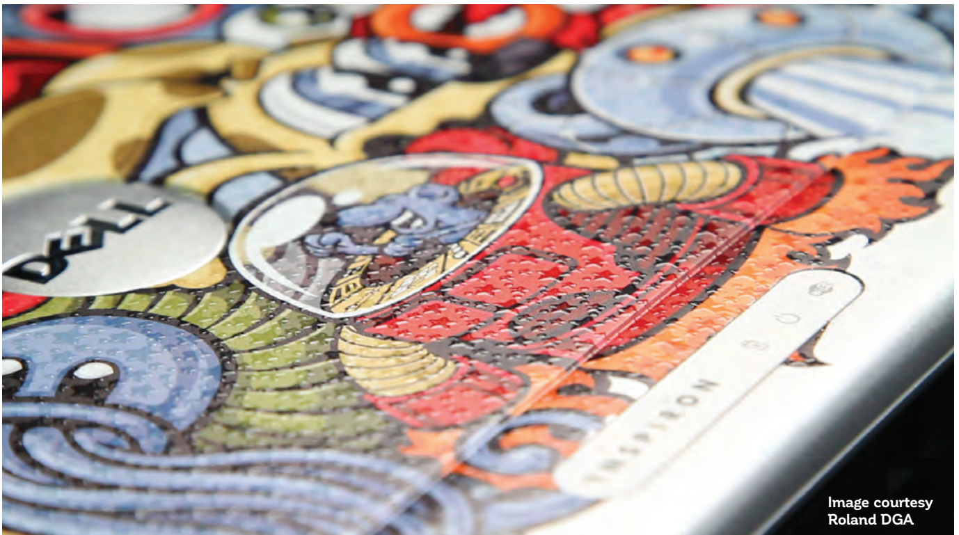
These printers can create different textures and even two-dimensional images using different drop sizes and layering. (Image courtesy Direct Color Systems)
