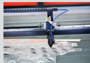
Lower-power CO 2 systems are extremely effective at marking and cutting wood, paper, acrylics, and many fabrics.
