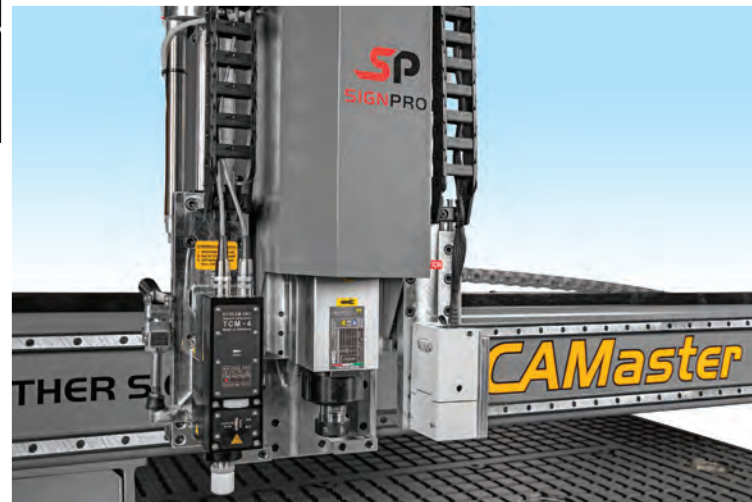
Most CNC routers can cut a variety of different materials from plastics like acrylic, polypropylene, and polyethylene to materials like foam, aluminum, non-ferrous metals, wood, and composites. (Image courtesy CAMaster)
