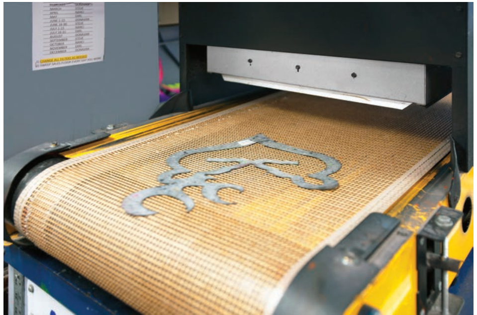
Once the infrared conveyor dryer reheats the adhesive on the stencil, Mark applies the stencil to the shirt and airbrushes finishing touches.
