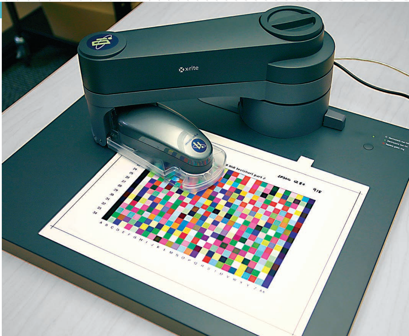
Fig. 2. A spectrophotometer is used to measure the color on a target print.
