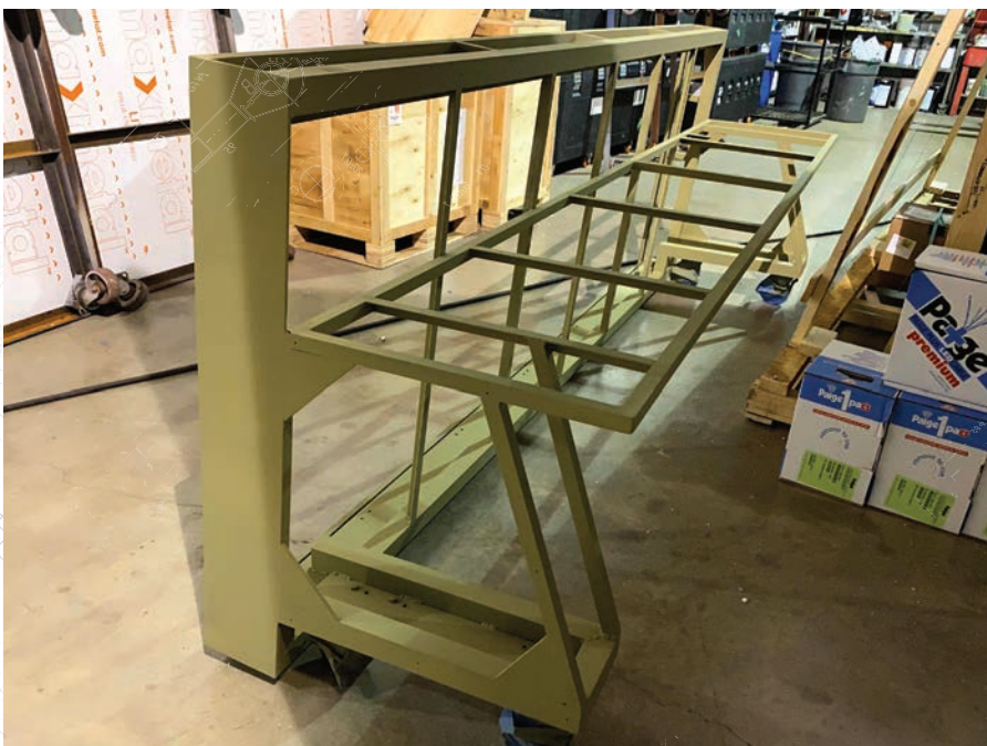
Once the frame has primer, it is prepped one last time for final finish.
