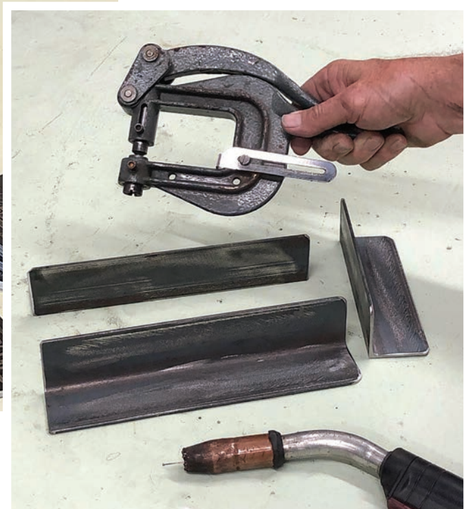
Above: Some of our best jobs are in making our smallest products, but the tedious job of hole punching in small tags and signs must be addressed. Right: We modify nearly all our sheet metal punches, and the basic modification is making a base for them so punching becomes a one-hand operation. (All images courtesy Rick Williams)
