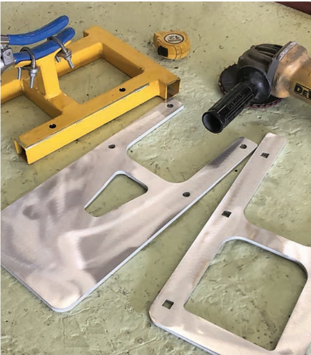
A tabletop to fit around the jaws of the punch, as well as a larger base plate, were made from .25" thick aluminum plate.
