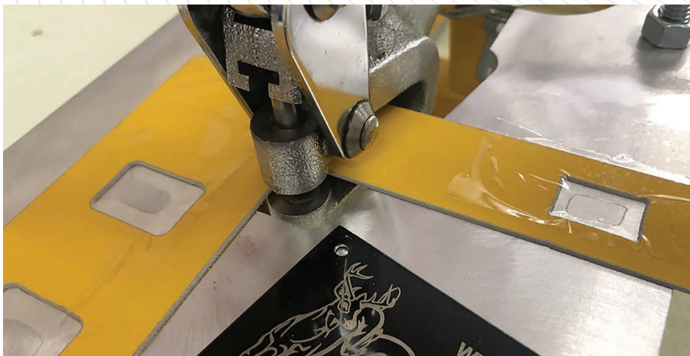
Once the exact location of the hole in a batch of tags is determined, a guide or stop (here made from yellow .040 aluminum) is taped in place until the job is done.
