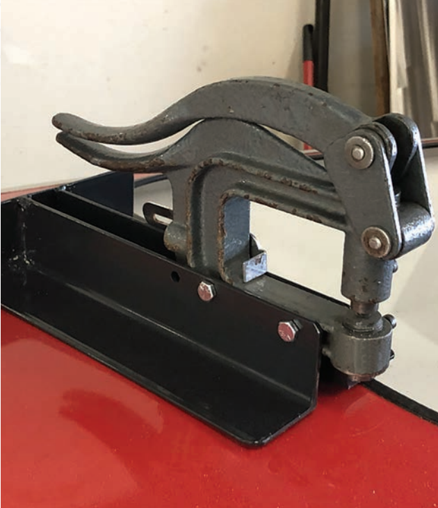
This base was constructed of just three pieces of 2" angle iron.
