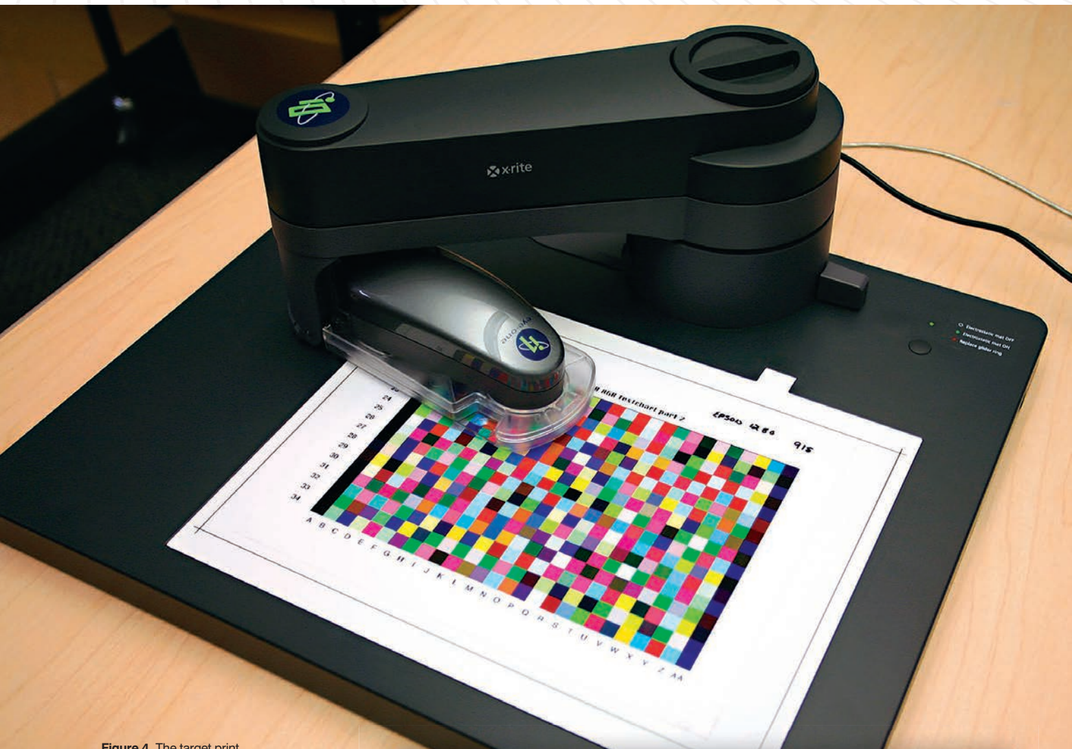
Figure 4. The target print is measured by a hardware device called a spectrophotometer.
