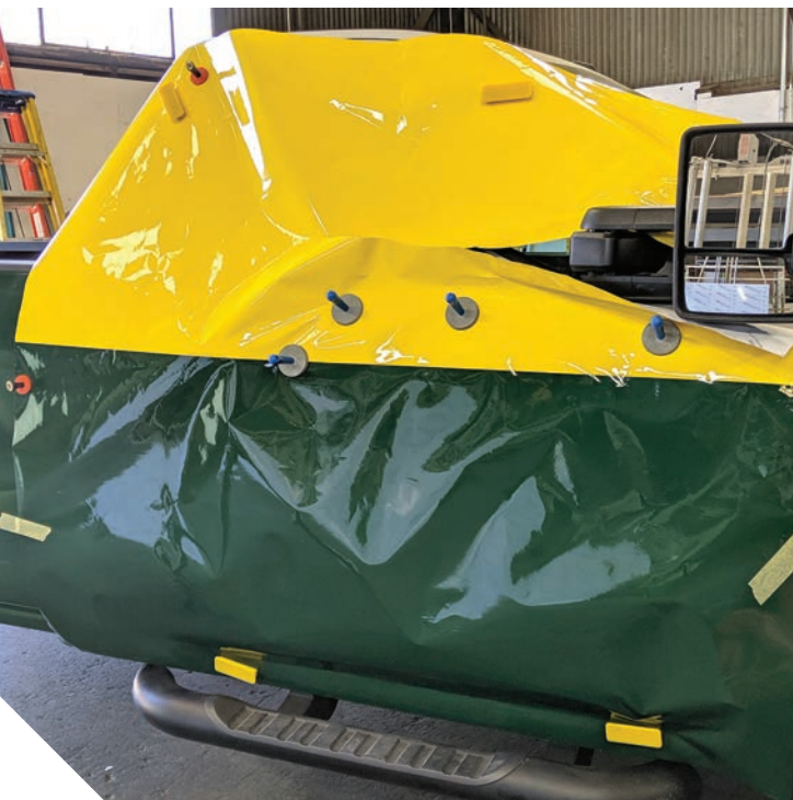
Above: We were provided the graphics for this install and they were a little short for the door, which meant a tight fit. We also had to maintain the horizontal line while working around the door handle and mirror. Careful placement and a relief cut around the mirror allowed us to stretch where needed while keeping the graphics in place. Right: The graphics are installed on this large hood, but all of the edges still need to be smoothed and the tension released before we do any trimming.
