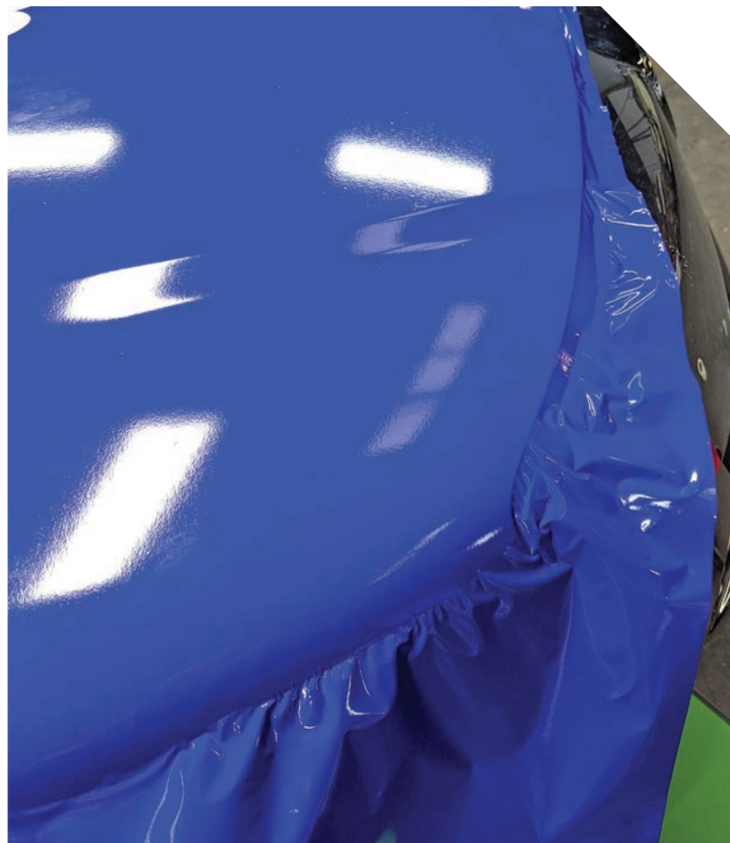
Above: We were provided the graphics for this install and they were a little short for the door, which meant a tight fit. We also had to maintain the horizontal line while working around the door handle and mirror. Careful placement and a relief cut around the mirror allowed us to stretch where needed while keeping the graphics in place. Right: The graphics are installed on this large hood, but all of the edges still need to be smoothed and the tension released before we do any trimming.
