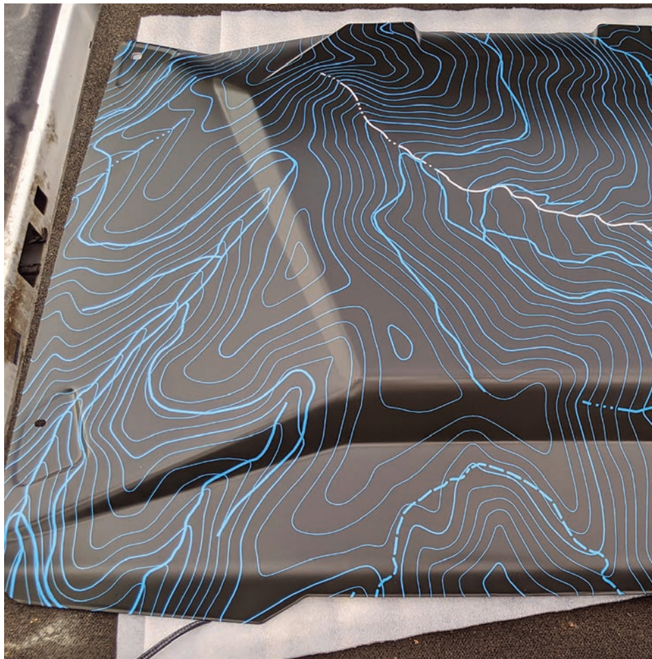
Above: The body lines on this full wrap included many curves and corners that required careful stretching and trimming for a clean finish. Right: This was a full wrap on the hood of a Can-Am Off-Road Side-By-Side. The contours are not extreme, but still require special attention to ensure a smooth finish. All corners and edges were also carefully stretched and post heated for long-term durability.
