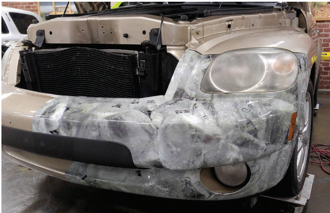
Learning to wrap the front bumper of an HHR during my 3M training brought together multiple techniques taught during the class. (All images courtesy Charity Jackson)
