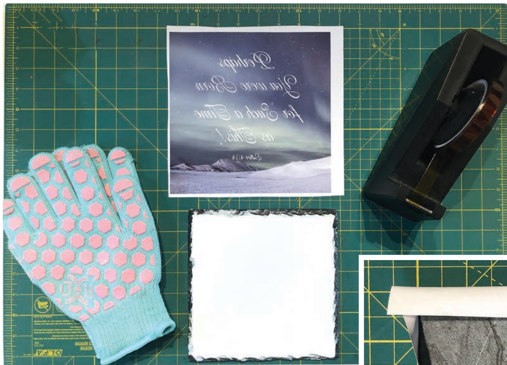
Left: The items needed to sublimate slate using the 3D vacuum press. Step three ( below ): the slate is placed face down and the image is secured with tape.
