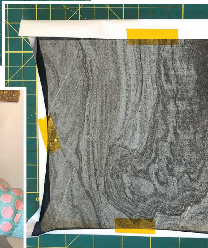
Left: The items needed to sublimate slate using the 3D vacuum press. Step three ( below ): the slate is placed face down and the image is secured with tape.
