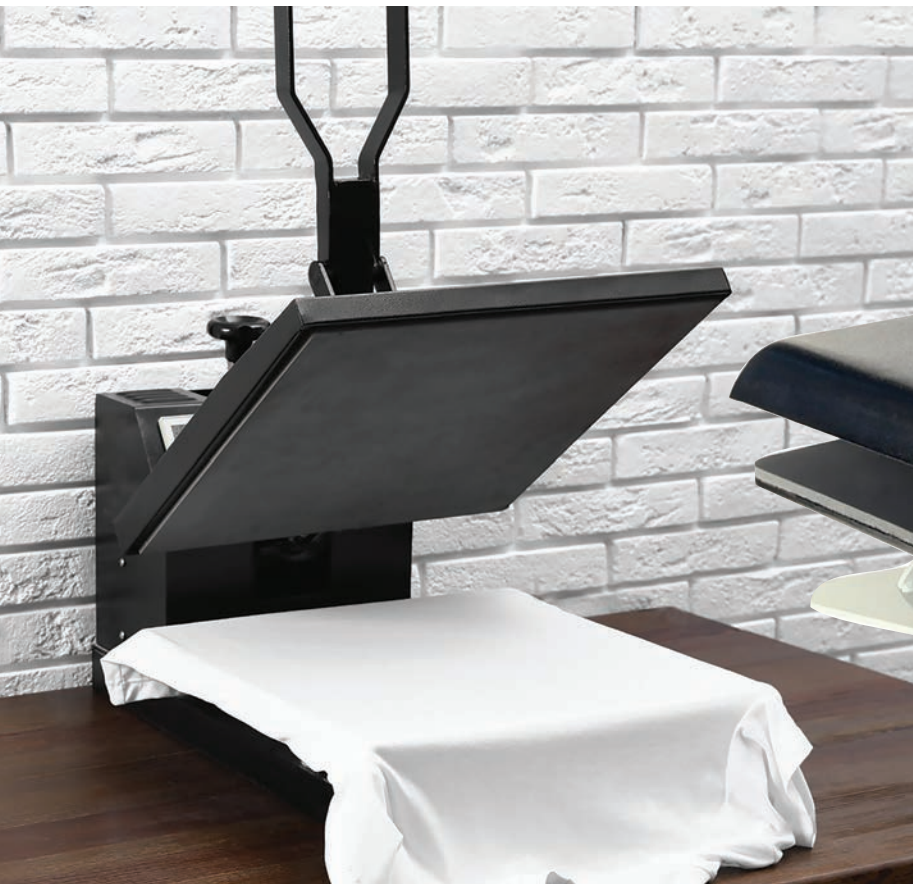
Above: Swing-away presses open and the top swings away entirely from the lower platen. Left: A clamshell heat press is ideal to operate in a small space. (All images courtesy Cheryl Kuchek)
