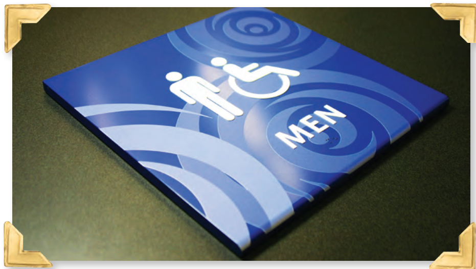
Clean, modern design for a restroom sign. It's a photopolymer sign leaving raised copy and Braille, painted first surface with non-glare paint. Copy and pictograph is "tipped," meaning white ribbon material is thermo-pressed on the raised surface. Photopolymer has been the standard for schools for decades. (Photo courtesy of Park Place Sign Systems)
